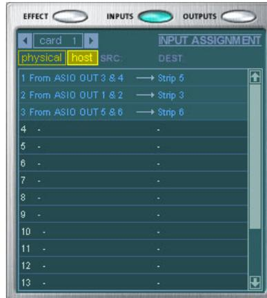
❖ **Tip:** Clicking on any of the input routings in the TV display highlights the corresponding mixer strip.
