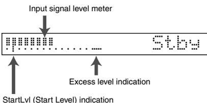
Turn the INPUT LEVEL knob on the rear panel with your eye on the level meter to maximize the input level within the range in which the excess level indication remains unlit.
