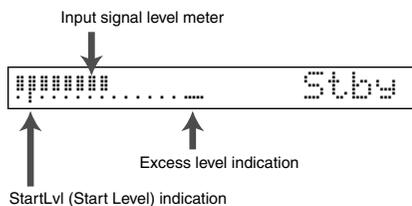
Turn the INPUT LEVEL knob on the rear panel and watch level meter to maximize the input level without lighting the excess level indicator.
