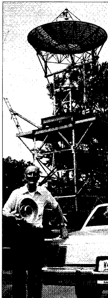
Fig 1—Paul Wilson, W4HHK, holds a 2304-MHz feed for his 17-foot Kennedy dish (background).
