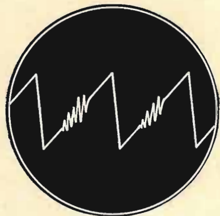
Fig. 5—Mysterious "squiggle" in horizontal oscillator waveform: power supply trouble.
