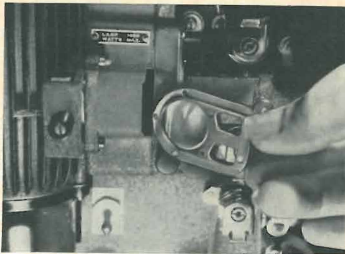
Fig. 6—Closeup of condenser lens, removable for cleaning. Other one is still inside, about 1 inch left of slot.
