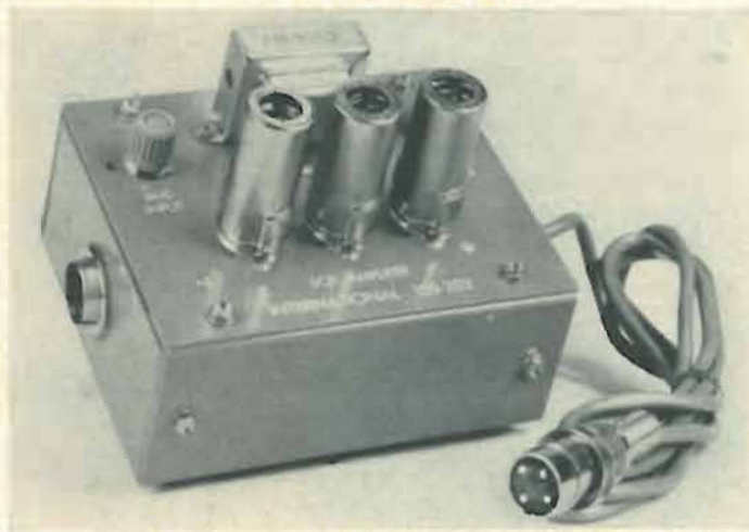
Fig. 3—Circuitry of International Crystal Executive speech clipper/filter amplifier (photo below). Sharp filter removes harmonics created in clipping process.
