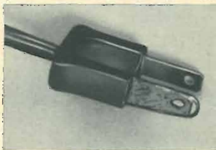
Handy trick for making polarized plug—solder paperclip over one prong. This prong goes to ground side of line. This plug fits modern wall receptacle. You can buy polarized plugs from most big electrical supply houses.
