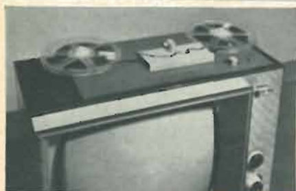
The video tape recorder measures 17½ x 9 x 6 inches and weighs 15 pounds. (Below) Recorder built in as part of a TV receiver.
