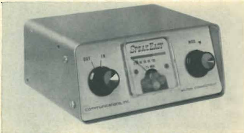
Fig. 5—"SpeakEasy" (below), another type of compressor, incorporates modulation percentage meter. High-level control signal comes from CB set's modulator.
