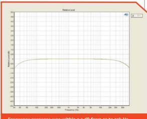
Frequency response was within 0.2 dB from 50 to 30k Hz.
