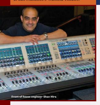
Front-of-house engineer Shan Hira is mixing on a Soundcraft Vi6, using all onboard effects except for a Manley Voxbox and an XTA 1/3-octave graphic EQ on Allen's vocals.
