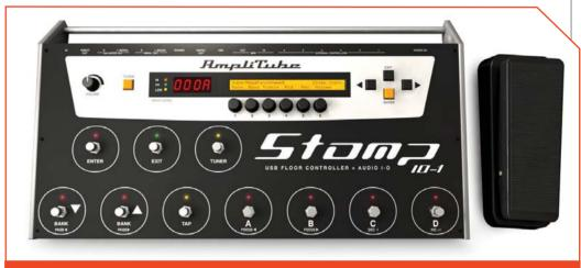
StompIO's interface supports up to six external controller inputs, including expression pedals and footswitches.
