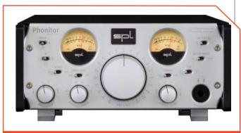
Phonitor's Crossfeed, Speaker Angle and Center Level controls provide ways to simulate a speaker's interaction with a room.
