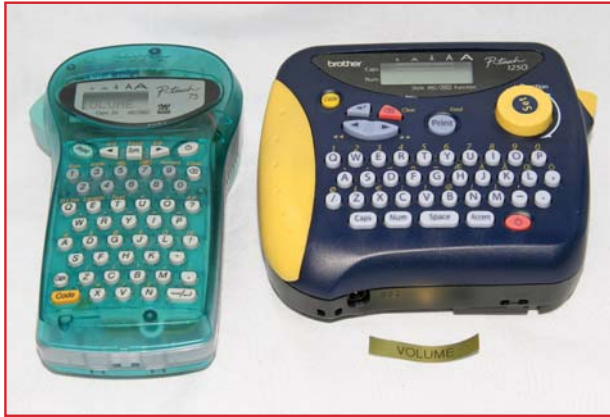
Fig.2. The smaller electronic labelling machines probably represent the simplest way of producing good quality panel legends. Tapes offering various combinations of text and background colour are available
