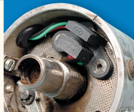
This photo shows how the slotted Hall effect sensor is rivetted to the vacuum advance plate inside the distributor.
