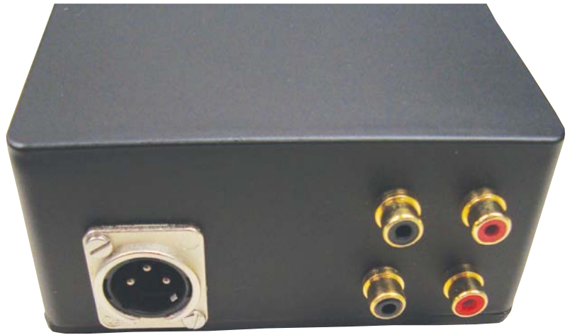
Rear view of the amplifier showing the pairs of phono sockets and the XLR chassis plug power connector
