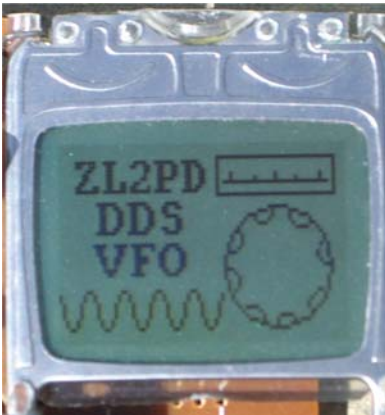
Fig.2: the readout, from a Nokia cellular phone, is capable of displaying simple graphics.
