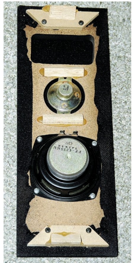
The woofer and cone-type tweeter are mounted on a front baffle, which is easily removed. Note the rather odd port design and the large gap around the tweeter!
