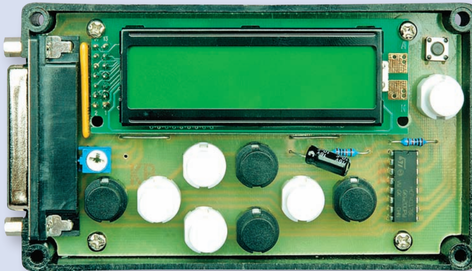
The PC board mounts inside the case on four M3 \times 12mm spacers and is secured using M3 screws, nuts and flat washers – see Fig.19. Note how the 10 \mu F capacitor is mounted on its side, so that it clears the front panel.
