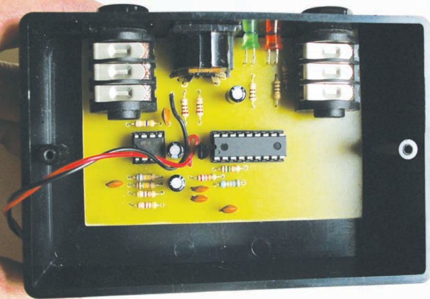
The completed circuit board mounted in its case. The plastic jacket socket mounting nuts hold the board firmly in place
