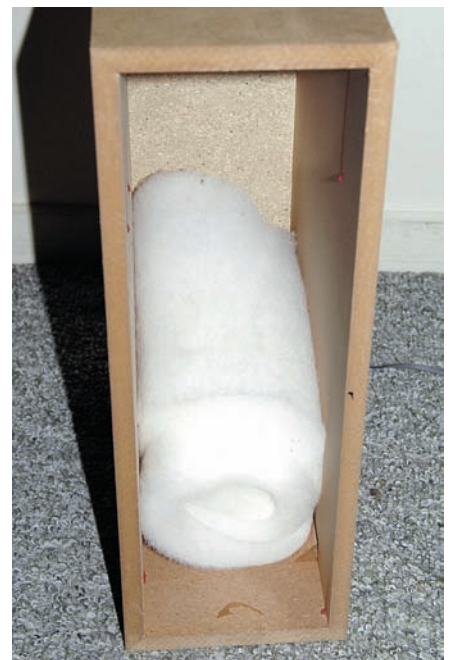
Another oddity was the internal box fill, which was rolled into a cylinder and placed at one end of the box (in front of the port?).
