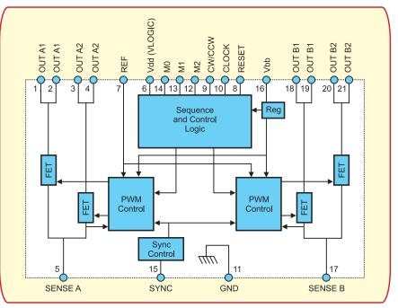
Fig.1: Simplified internal block schematic and functional diagram for the SLA7062M stepper motor translator/driver IC
