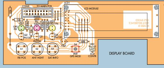
Fig.6(b): assemble the display PC board as shown here. Switches S1 to S3 must be mounted with their flat sides as shown, while LEDs 1 to 3 should sit 11mm above the board surface. Note also that the 10µF capacitor must be mounted flat against the board (see photo).
