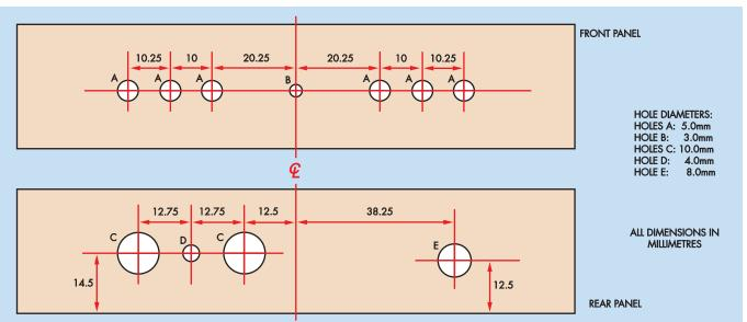
Fig.10 (above): these are the drilling diagrams for the front and rear panels of the transmitter case. They can be photocopied or downloaded from our website and directly used as drilling templates if required.
