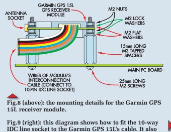
shows how to make the 16-way IDC ribbon cable.
