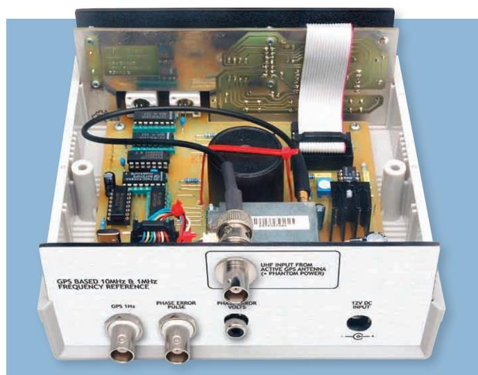
The rear panel carries BNC sockets for the antenna (top, centre) and for the GPS 1Hz and phase error pulse outputs (bottom left). It also carries an RCA phono socket for the phase error voltage and provides access to the DC power socket.
