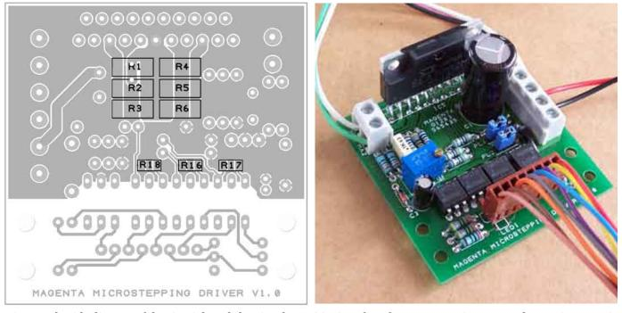
Fig.4: Underside diagram of the circuit board showing the positioning of 'surface mount' resistors. Speed-up resistor R16 is necessary for high stepping rates, but R17 and R18 will not be required in most applications. The completed Microstepping board is shown above. The 'thermal tab' of IC5 will probably need a small heatsink attached to it – see text
