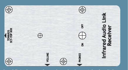
Fig.9: these full-size front panel artworks can be photocopied and applied to the front and rear panels of the transmitter and to the lid of the receiver. Use wide strips of self-adhesive film to protect them from damage – see text.
