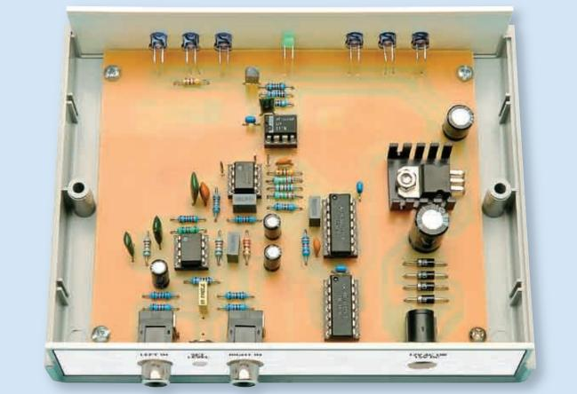
Here's another view inside the completed transmitter. Note the lead dress on the infrared LEDs and the green indicator LED, so that they protrude through their matching holes in the front panel.
