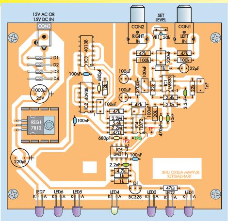
Fig.7: install the parts on the transmitter board as shown here, taking care to ensure that all polarised parts are correctly orientated. Below is a full-size photo of the assembled PC board.
