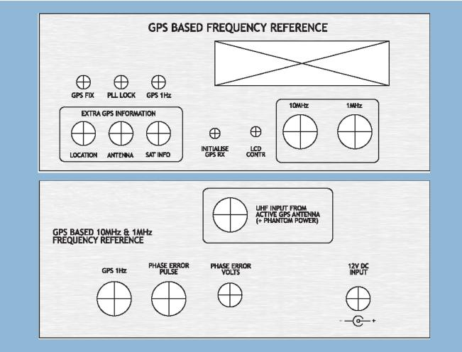
Fig.12: these full-size artworks can be copied and used to make the front and rear panels.
