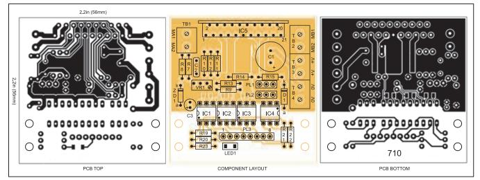
Fig.3. Stepper motor driver printed circuit board component layout and full size copper foil masters for the topside and underside of the board
