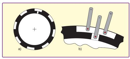
Fig.4. Incremental encoder for motion sensing (a) disc pattern, (b) sensor locations
