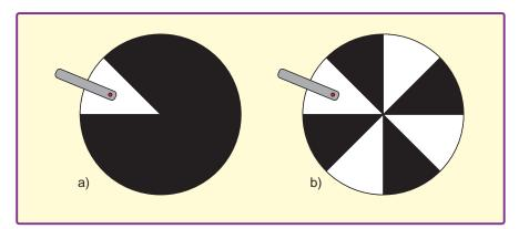
Fig.1. Optical sensing of motion
