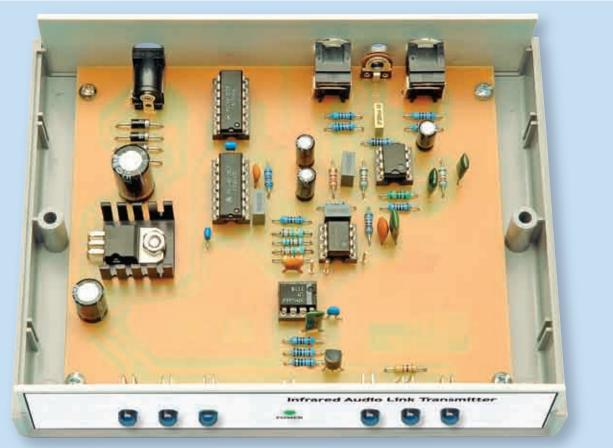
The completed transmitter PC board is installed in a low-profile instrument case and secured using four selftapping screws that go into integral mounting posts in the base. We used IC sockets for the prototype, but you can solder the ICs directly to the PC board.
