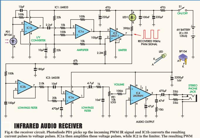
signal from the limiter is then fed to low-pass filter stages IC3b and IC3a and finally to audio amplifier stage IC4.
