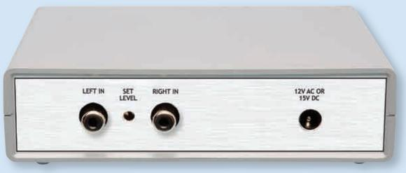
The rear panel of the receiver has clearance holes for the two audio input phono sockets, plus access holes for the 'Set Level' trimpot and the power socket. Power can come from a 12V AC or 15V DC (regulated) plugpack.
