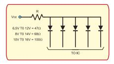
Fig. 8.4. When using a higher supply voltage, insert a resistor in series with the LEDs
