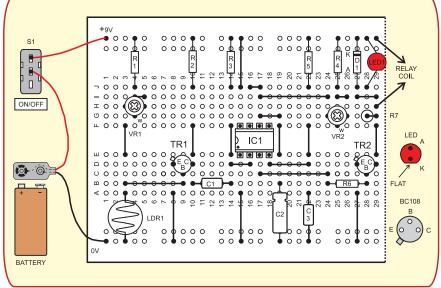
Fig.8.2. Motion Detector breadboard component layout
