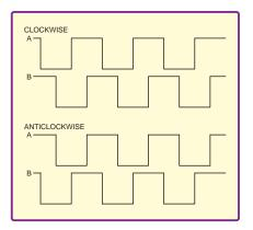
Fig.5. Quadrature signals from the incremental encoder shown in Fig.4a, starting from sensor positions shown in Fig.4b (With logic 0 for black and logic 1 for white)
