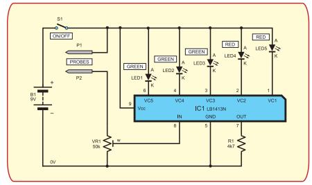
Fig. 8.3. Circuit diagram for the Moisture Monitor Mk.2
