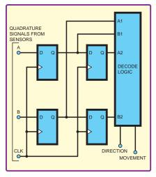
*Fig.6.* Quadrature decode circuit to determine direction of movement
