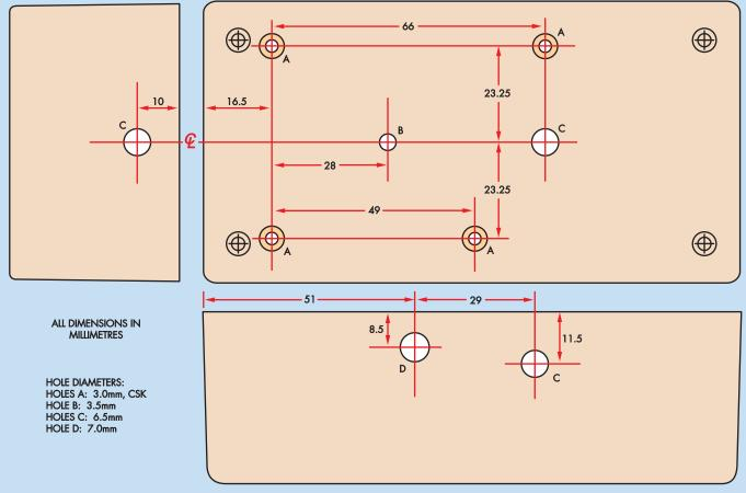
Fig.11: here are the drilling details for the receiver case. It's important to get all holes in their correct locations, so that everything lines up correctly when the receiver board is installed.
