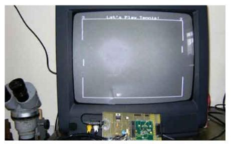
Fig.3. Example of TV display using the circuit in Fig.2.
