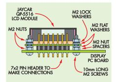
Fig.10: the LCD module is secured to the display board with M2  $\times$  10mm screws, nuts and flat washers.
