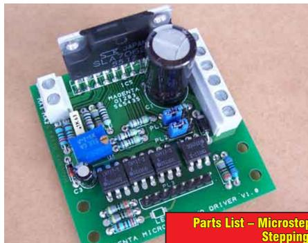
Two resistors, R7 and R8 have been used to allow for higher power dissipation, and to make it easier to use other resistance values to accommodate different motor supply voltages. The combined resistance value should be chosen to deliver 12mA at the nominal motor supply voltage.
