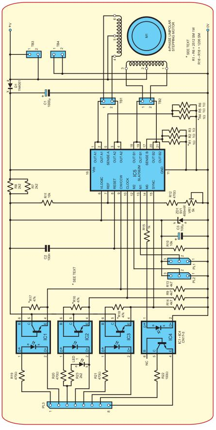
Fig.2: Full circuit diagram for the Microstepping Four-Phase Unipolar Stepping Motor Driver. LED 1, resistors R1 to R6 and R16 to R18 are surface mount types
