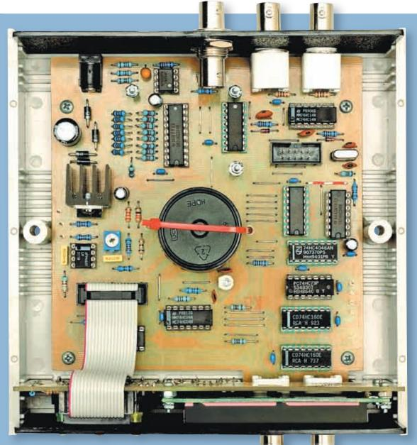
The main PC board is secured to integral spacers on the base of the case, while the display board slides into one of the case slots. Note that the front and rear panels must be attached to the BNC sockets on the main board before mounting it in the case.
