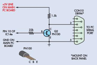
Fig.1: a serial data output port can be added to the GPS-Based Frequency Reference using this simple circuit.
