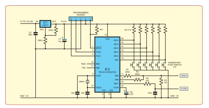
pins you wish. While it's not a particularly useful feature for us – ours is a very simple design that can be laid out on stripboard – it's great for those more complex designs where PCB layout requirements call for short or conveniently routed tracks.
