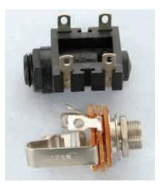
Fig.2. An insulated jack socket (top) and an open construction stereo type (bottom). Unlike open construction sockets, the insulated type does not provide a connection to the panel via the body of the component
