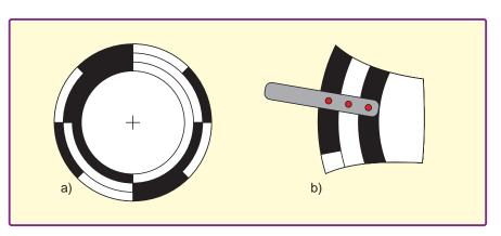
Fig.2. (a) Disc patterned with binary code, (b) arrangement of sensors
