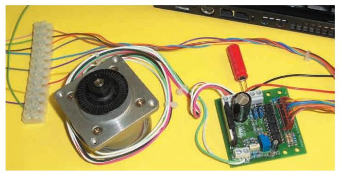
The completed circuit board linked to a small 200 step motor. Note the motor decoupling electrolytic capacitor wired directly between terminal blocks TB3 and TB4. It should have a *minimum* value of  $470\mu$ F, see text
