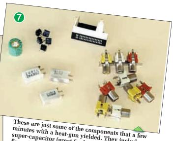
muse are just some of the components that a few minutes with a heat-gun yielded. They include a 0.22F super-capacitor (great for human-powered LED torches), five micro pushbutton switches, a 2-channel LED bargraph display, nine RCA phono sockets and three high-power resistors. Not shown are the 20 electrolytic
