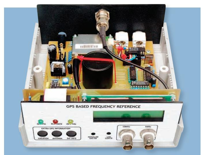
This view shows the fully-assembled unit, with both the Garmin receiver and the oven cover in place. Note the internal antenna connection from the Garmin GPS 15L receiver's socket to the BNC-to-BNC adapter on the rear panel (see also picture on facing page).
