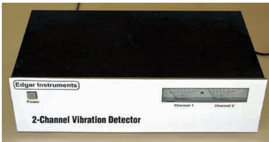
It looks like a £1000 instrument but costs less than £5 to make. This 2-channel vibration detector is actually based on a slightly modified cassette deck and uses conventional loudspeakers as vibration sensors. It's sensitive enough to detect a cat walking past on a wooden floor.
