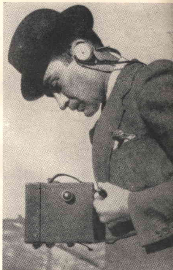
Fig. 5. A "midget" radio was one small enough to fit a (large) camera case.
