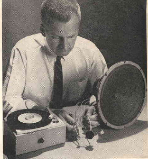
Molecular electronic phono system. Preamp is tiny unit in engineer's right hand, and 5-watt 0-20,000 cps power amplifier to drive speaker is in small black box in left hand.
