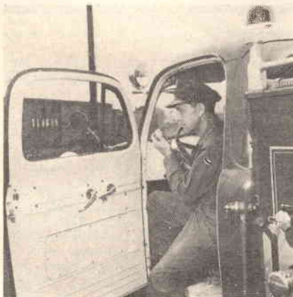
Fig. 5. This is a radio-linked fire truck. Other such vehicles include an ambulance, plant protection patrols, messengers, and mobile service trucks.
