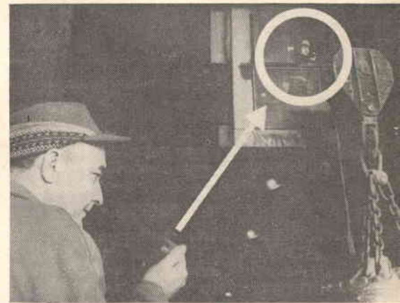
Fig. 6. A floor man guides the operator of the cab in an overhead crane in the steel mill through carrier-current radio. Hand signals are taboo.
