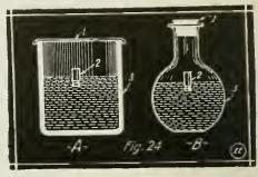
Apparatus With Which the Principle of the Submarine Can Be Demonstrated. The Small Vial 2, Can Be Made to Perform Many Wonderful Tricks By Pushing Down on Diafram 1, or Squeezing Bottle 3 in "B".
