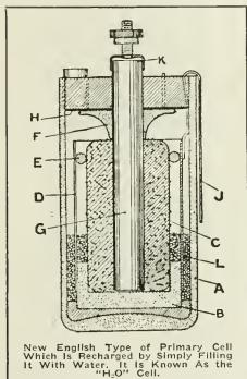
the demand for a wet cell smaller and more compact than the "Leelanché," and in this respect it appears to have gained its ad-vantage. This cell may be stored for any vantage. This cell may be stored for any length of time and in any climate without any deterioration. It is not liable to creeping or evaporation while in use. Its internal resistance is low, and it does not polar-
