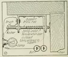
A Rellable Automatic Switch for Closet Light. When Door Opens the Switch Rod Is Moved Forward by the Spiral Spring as Be-comes Evident, and Vice-versa.
