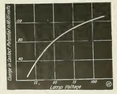
ve Showing Relation Between Light on Selenium and the Contact Potential.
