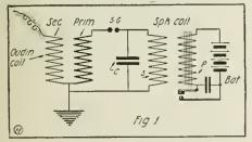
Fig. 1. Proper Connections for Small "Oudin" High Frequency Coil Excited by a Spark Coil or Step-up A.C. Transformer.
