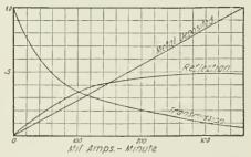
Fig. 2. Curves Showing Reflecting Power at 45 Degrees Incidence and Percentage of Metal Deposited and Light Transmitted for Platinum-iridium Mirror With Varying Prod-ucts of Time and Current.
