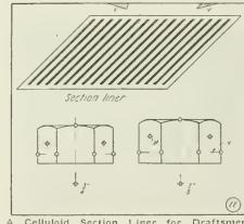
A Celluloid Section Liner for Draftsmen and a Scheme for Quickly Drawing Nuts or Bolt-Heads of Any Size.
