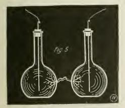
Startling Experiment With Two Glass Water Bottles Connected to Tesla Coll. The Spark Jumps Between the Glass Surfaces and Illuminates Solutions Within the Bottles.
