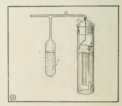
Arrangement of Apparatus for Measuring Pressure of Light.—H is Hollow Stopper, E Is Cover Glass Cemented to Tube, F Con-tains Pith Charcoal, G Is Tube Which May Be Connected to Gaide Pump.
