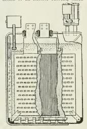
is caused to flow there-thru from one electrode to another, both electrodes being submerged in water. The solution is decomposed in the well-known electrolytic manner, oxygen being liberated at the positive electrode and hydrogen at the negative electrode. This invention relates particularly to an electrolytic gas generator in which the liquid acted upon is contained in a suitable receptacle, having two sets of insulated electrodes entirely independent of the receptacle proper.
