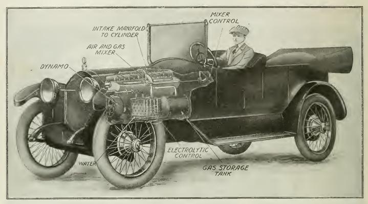
A Detroit Genius Claims to Have Solved the "Gasoline Substitute" Problem for Automobiles. He Utilizes a Very Simple Electrical Phenom-enon—That of "Electrolysis" or the Decomposition of Water by the Passage of An Electric Current Thru It. The Hydrogen Gas Evolved Is Mixed With Air and Past Into the Engine Cylinders. The Inventor States That It Is More Economical Than Gasoline Because of the Higher Explosive Value of the Hydrogen-Air Mixture.
