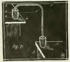
Demonstration and Controlling Factors of the Hydrostatic "Siphon". A Simple and Effective Method of Emptying Tanks and Even Reservoirs When Occasion Requires It.
