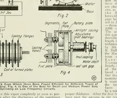
Various Styles of Radio Spark Gaps Which Have Been Found Efficient for Different Types of Sets. The Rotary Quenched Gap, Fig. 4, Is One of the Best for Small and Medium Power Sets Operating on Low Frequency Circuits.
