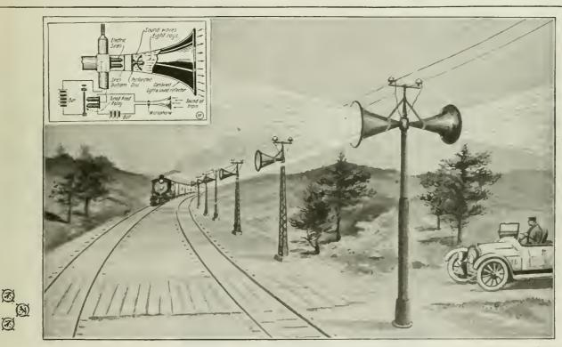
Instead of Having the Gateman Sound the Alarm at Railroad Crossings This Inventor Proposes That Sensitive Microphones be Erected Along the Crossing Approaches, the Sound of the Locomotive's Whistle Causing Them to Actuate a Relay Device Connected to an Automatic Crossing Signal.
