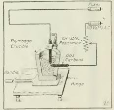
A Simple "Arc" Furnace Made From Two Carbon Rods and a Plumbago Crucible.
