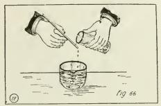
Method of Pouring Small Quantities of Acid onto a Glass Rod so That They Drop into a Beaker or Other Dish Easily.
