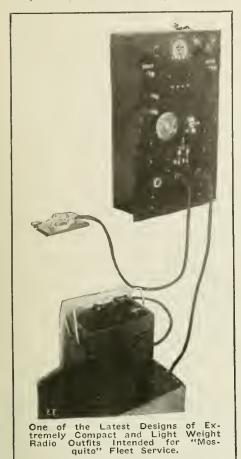
a current derived from a storage battery. It was designed for supplying the mosquito fleet with an efficient low power transmitting outfit.
