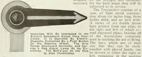
This, like other inventions of Mr. Hartman, is really quite simple in construction and performs its functional duty just as well, or perhaps better, than many existing and more complicated similar devices. The sole purpose of this instrument is to warn an automobilist in which direction the machine ahead of him is going to turn, either
