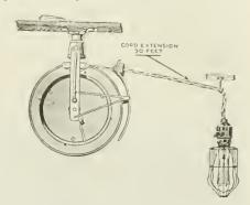
A Clever Invention in the Form of An Automatic Extension Reel for Portable Electric Lamps, Which Winds the 30-foot Cord Up and Swivels In Any Direction.
