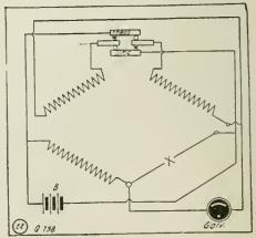
How a Reversing Key Is Connected in a Wheatstone Bridge.
