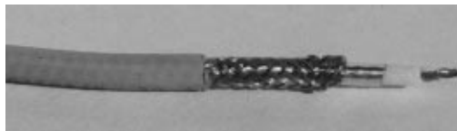
Fig. 3.19 - Cavo Thin Ethernet.
