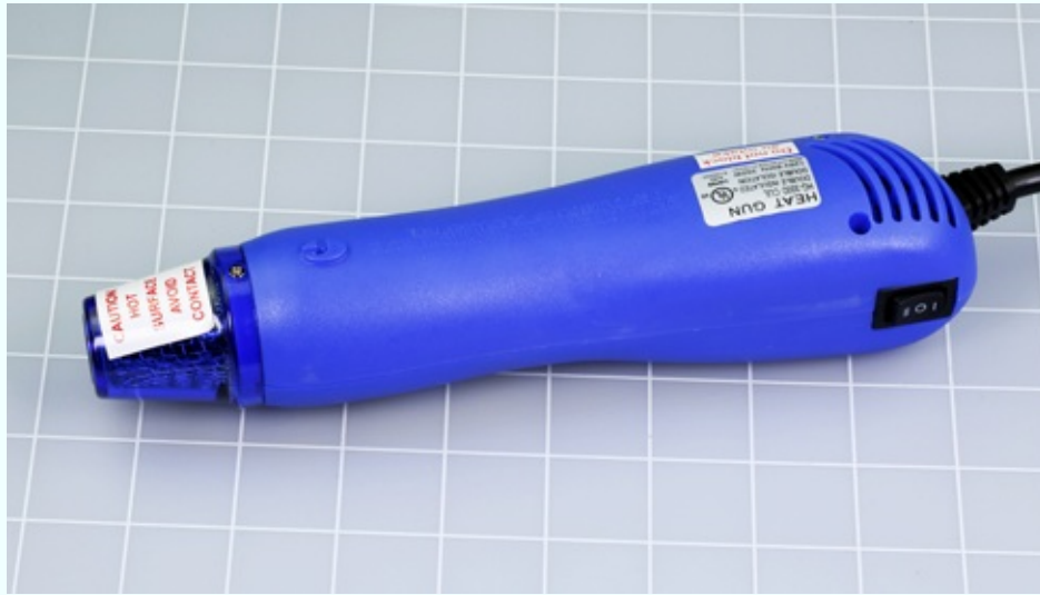
Figure 3-11. A miniature heat gun is slightly easier to handle than the full-sized type.
