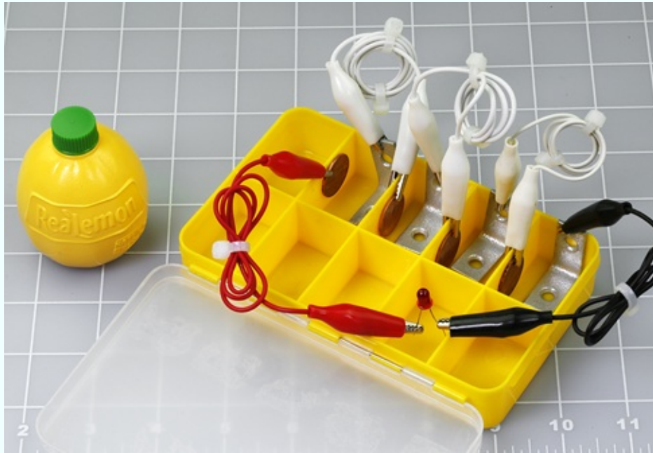
Figure 1-65. Lemon juice, either from lemons or from a squeeze-bottle, will produce reliable results, even though the equipment doesn't look so nice. Here a box intended for parts has been repurposed as a four-cell juice battery.
