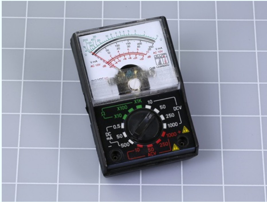
Figure 1-1. This kind of analog meter is inadequate for your purposes. You need a digital meter.
