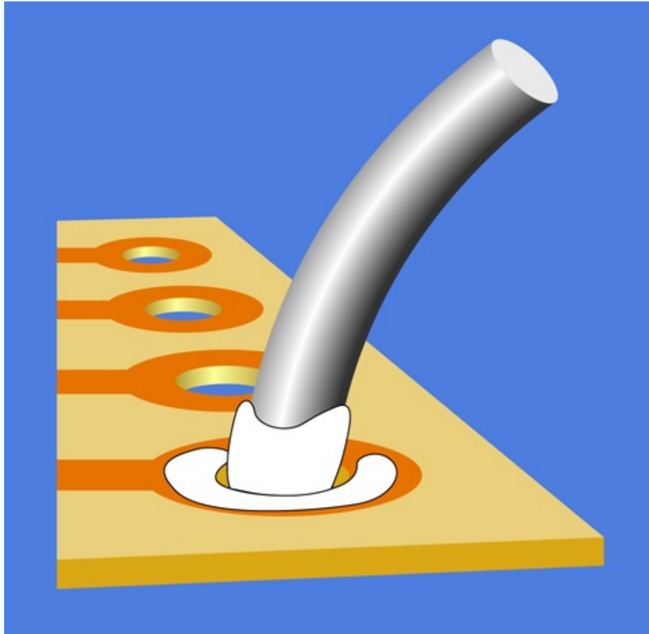
Figure 4-54. Too little solder (or insufficient heat) can allow a soldered wire to remain separate from the soldered copper on the perforated board. Even a hair-thin gap is sufficient to prevent an electrical connection.
