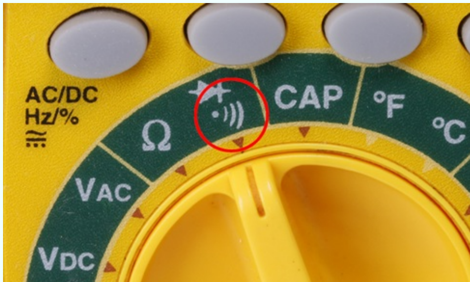
Figure 2-34. Another meter dial set to measure continuity.
