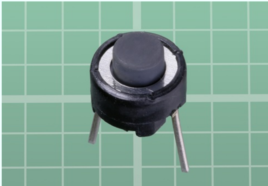
Figure 2-19. The recommended tactile switch for breadboarded projects in this book.
