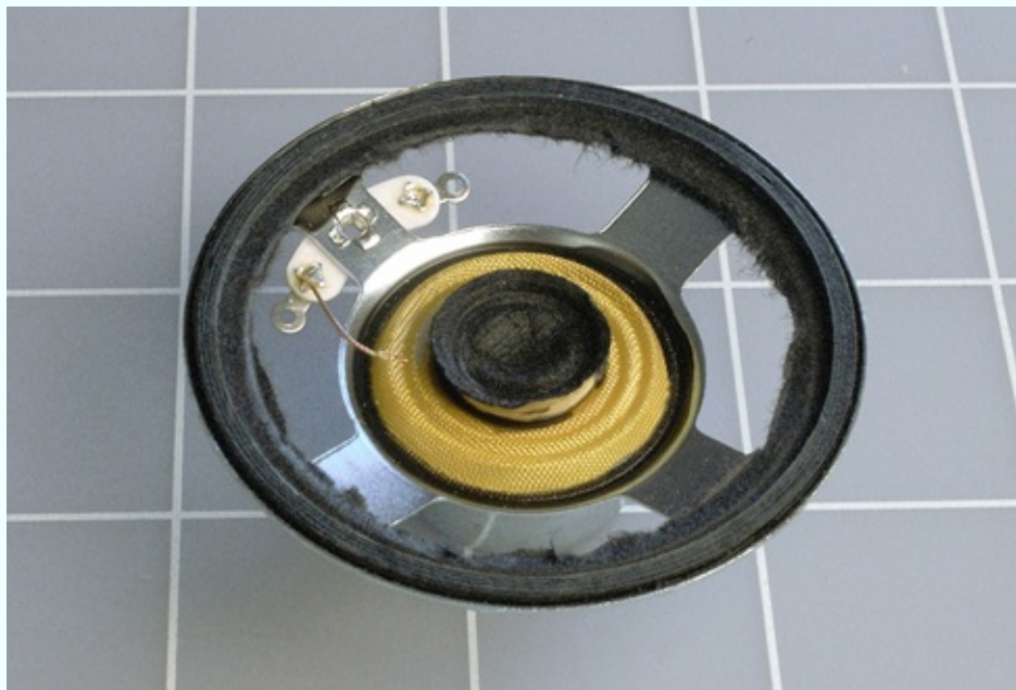
Figure 5-27. The loudspeaker with its cone removed.
