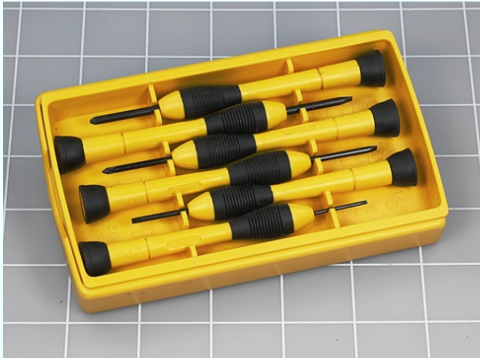
Figure 2-1. Miniature screwdrivers, with both flat blades and Phillips blades. The white lines are spaced at intervals of 1”.
