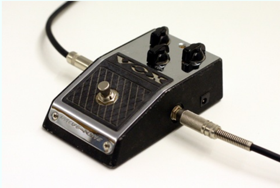
Figure 5-60. This Vox Wow-Fuzz pedal was one of the early stomp boxes, which deliberately induced the kind of distortion that audio engineers had been trying to get rid of for decades.
