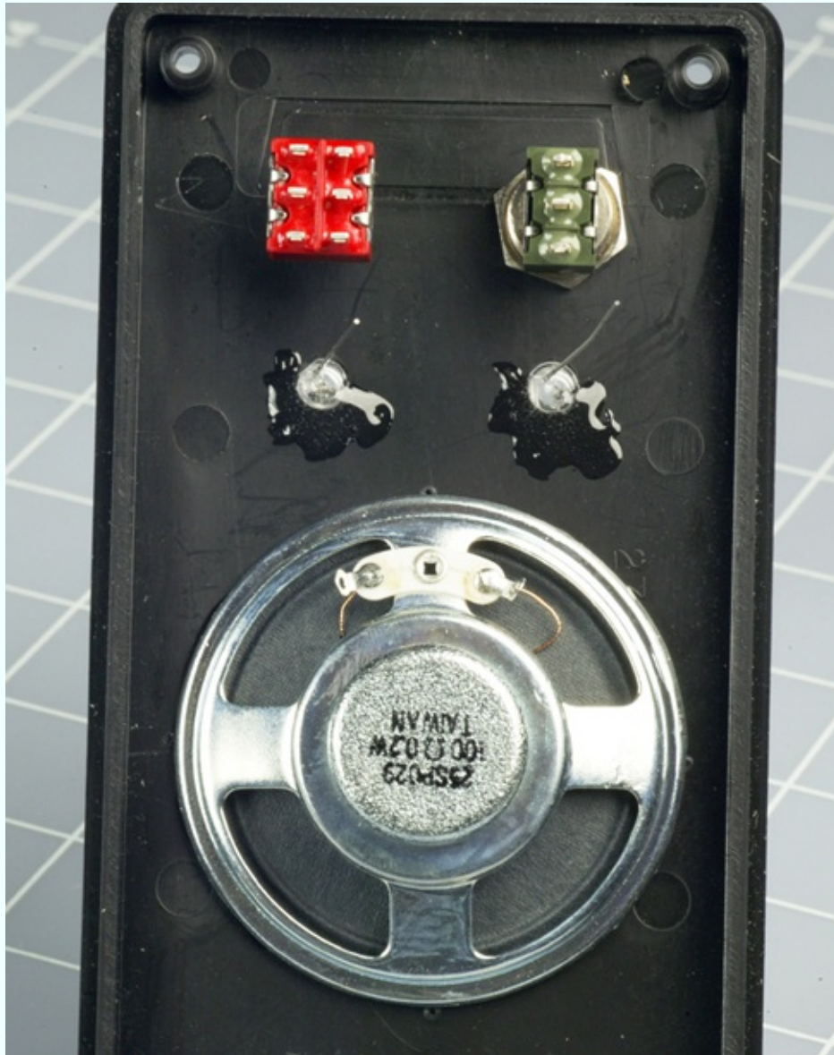
Figure 4-57. Components have been added to the control panel of the project box (seen from the underside). The loudspeaker has been glued in place. Spare glue was dabbed onto the LEDs, just in case.
