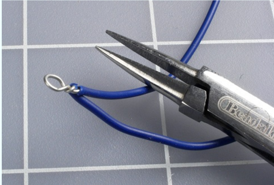
Figure 5-67. Create a loop in the section of wire that you exposed.
