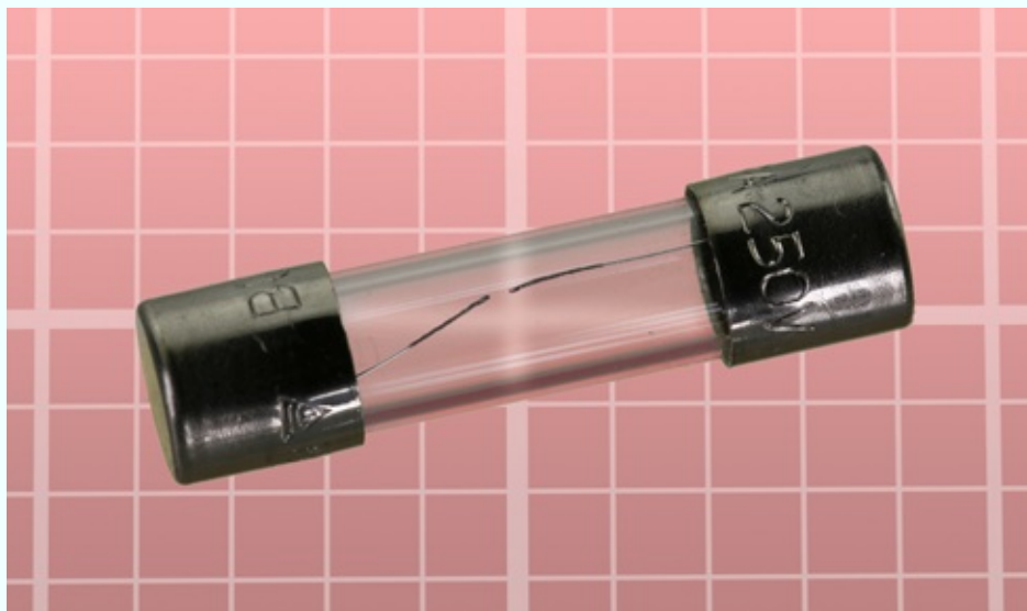
Figure 1-38. In a shorted cartridge fuse, a similar break appears.
