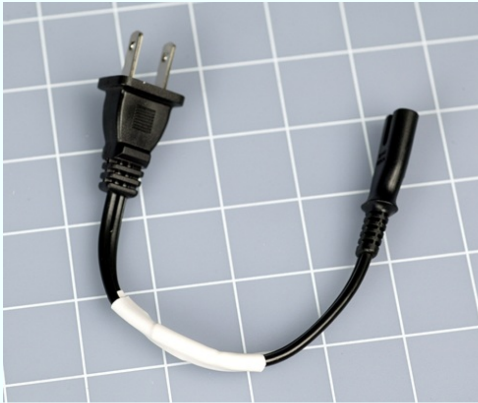
Figure 3-61. The power cord, shortened.
