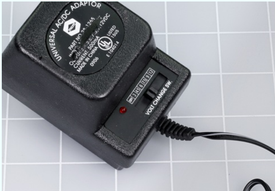
Figure 3-1. This AC adapter plugs into the wall and allows you a choice of DC voltages by moving a small switch.
