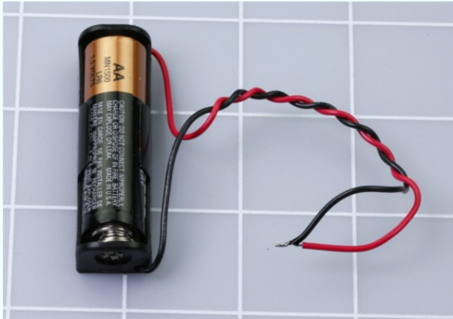
Figure 1-30. Shorting out an alkaline battery can be safe if you follow the directions precisely.
