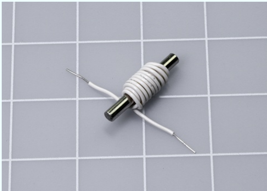
Figure 5-17. Adding more turns of wire will increase the measured voltage when the magnet moves through them.
