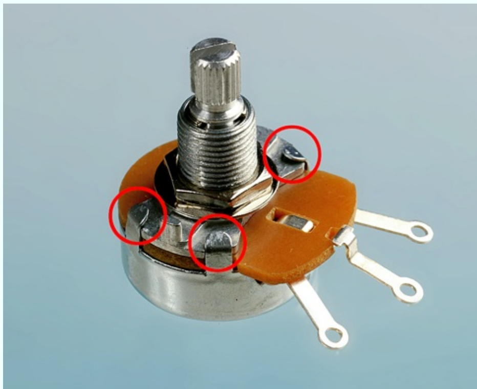
Figure 1-48. The tabs that hold a potentiometer together.
