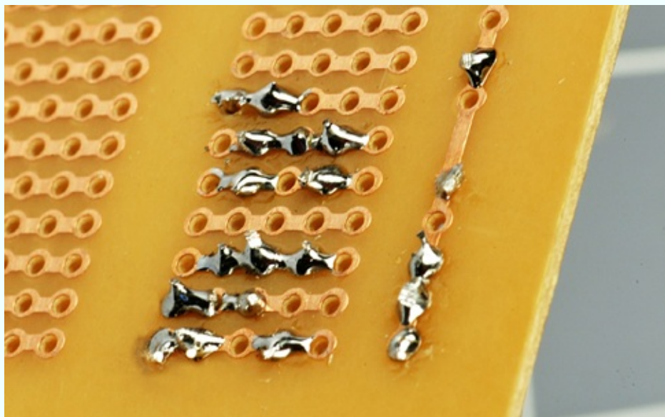
Figure 4-52. After soldering, the leads are snipped short and the joints are inspected under a magnifying glass. Another two or three components can now be inserted, and the process can be repeated.
