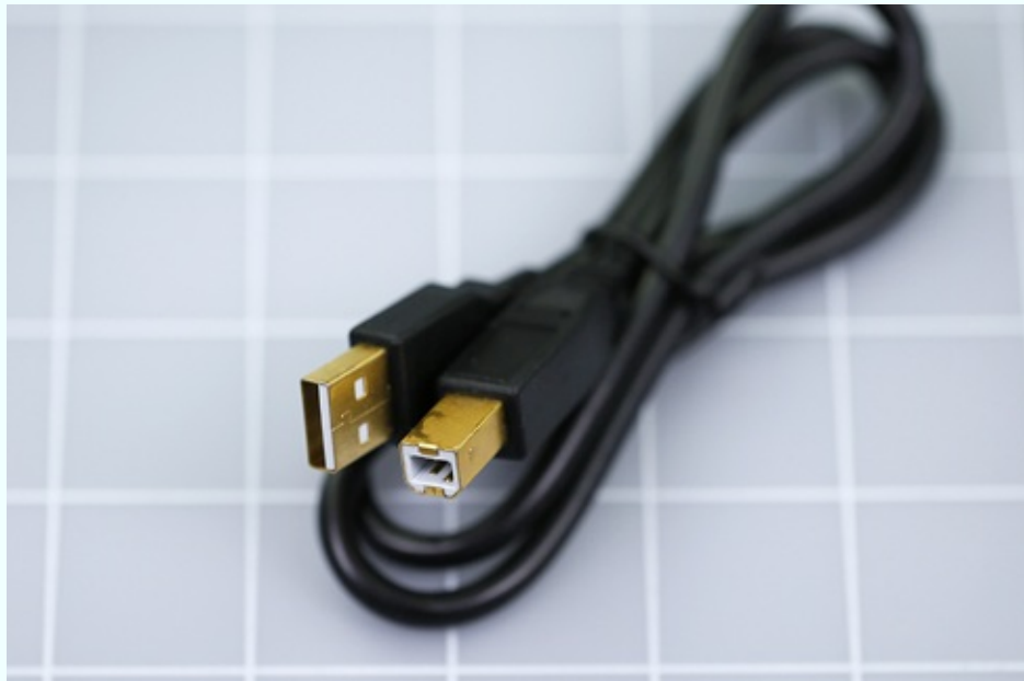
Figure 5-81. You will need this type of USB cable to attach your Arduino board to a USB port on your computer.
