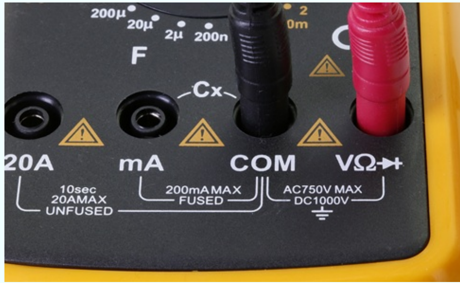
Figure 1-20. Sockets on one more meter.
