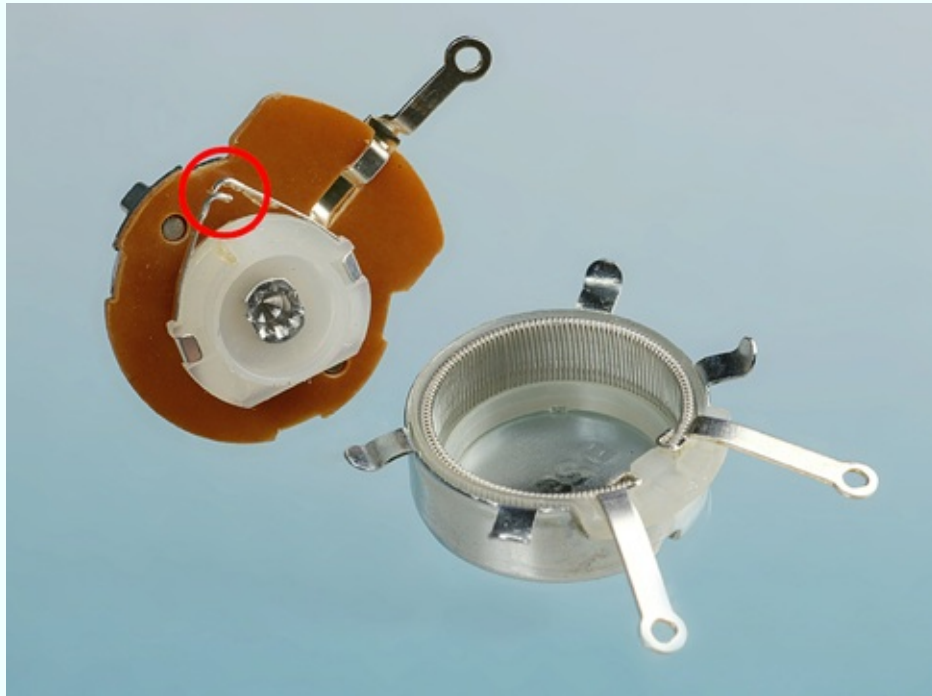
Figure 1-50. The wiper of the potentiometer is circled.
