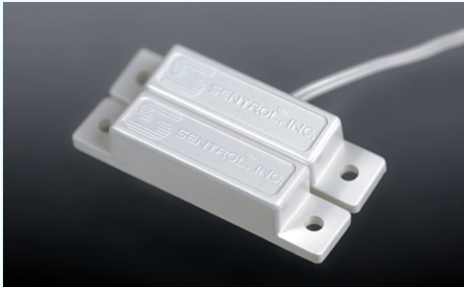
Figure 3-75. A typical alarm sensor consists of a magnet in a plastic pod (bottom left), and a magnetically activated reed switch in a similar pod (top right).
