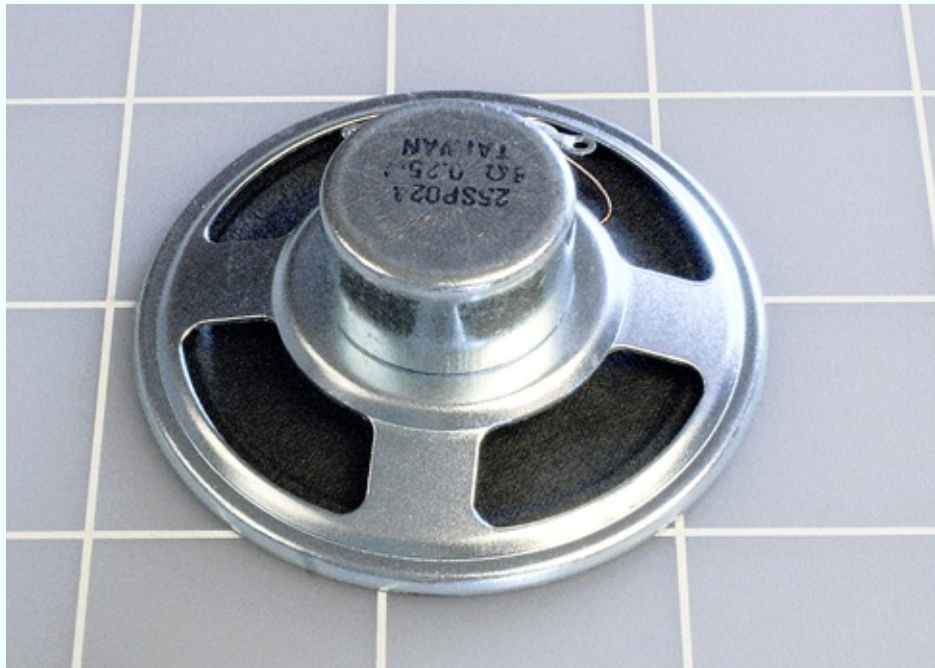
Figure 5-25. The back of a small loudspeaker.
