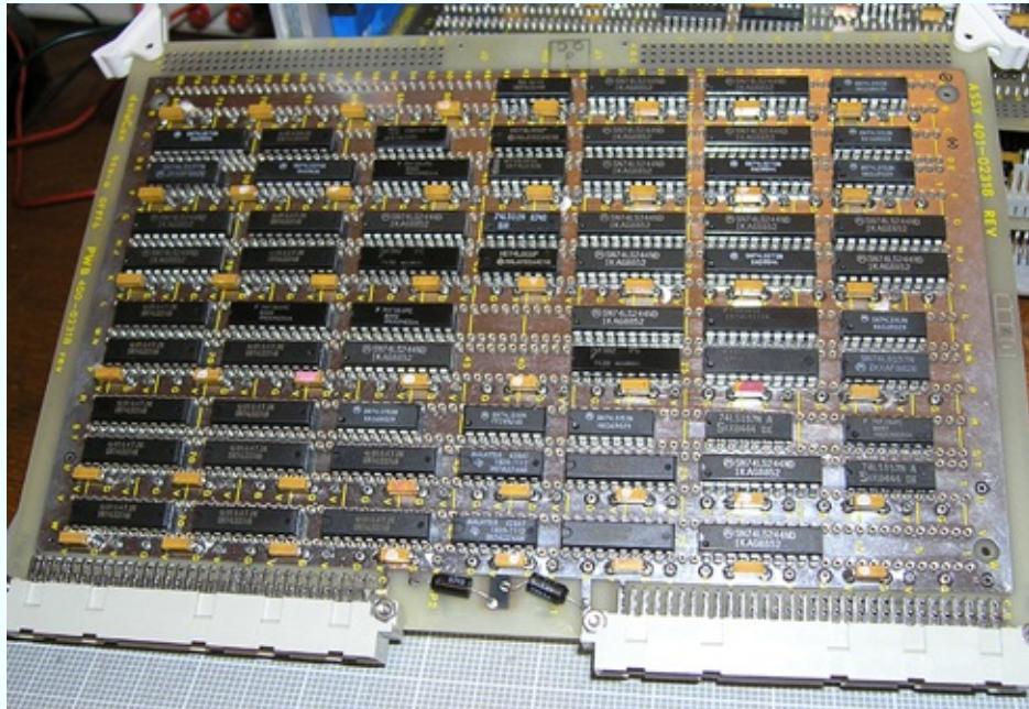
Figure 4-84. This computer motherboard hand-made by Bill Buzbee is built from 74xx series logic chips, and functions as the hearts of a web server.
