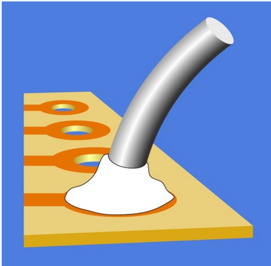
Figure 4-49. Ideally, your solder joint should look something like this.
