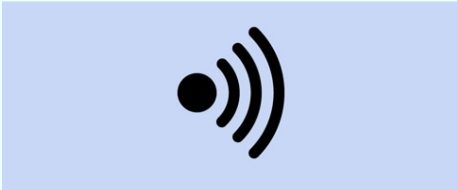
Figure 1-7. This symbol indicates the option to test a circuit for continuity, with audible feedback. It's a very useful feature.
