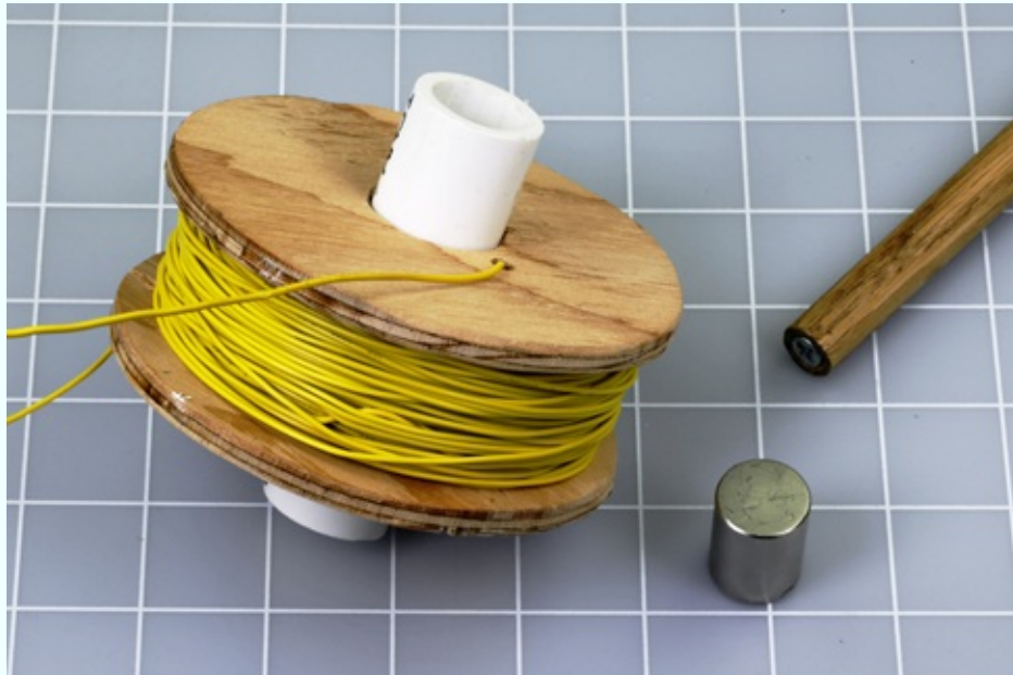
Figure 5-18. Two hundred turns of 22-gauge wire on a home-made spool, with a magnet that attaches itself to a screw in a wooden dowel.
