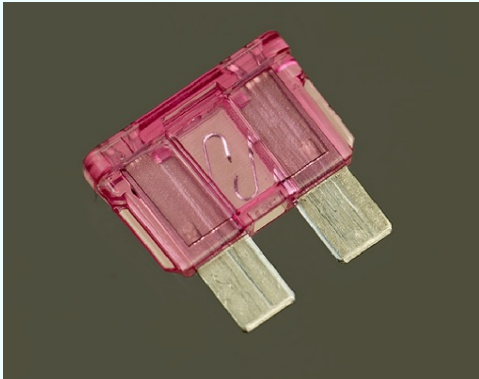
Figure 1-37. Note the break in the element.
