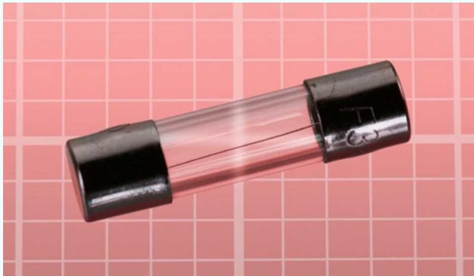
Figure 1-13. You can use a cartridge fuse like this, although your alligator clips won't grip it so easily.
