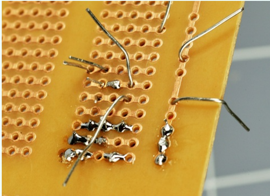
Figure 4-51. This photograph was taken during the process of transferring components from breadboard to perforated board. Two or three components at a time are inserted from the other side of the board, and their leads are bent over to prevent them from falling out.
