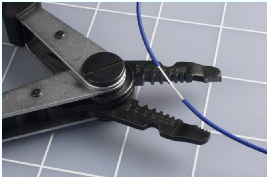
Figure 5-66. Use your wire strippers and your thumbnails to pull back about half an inch of insulation.
