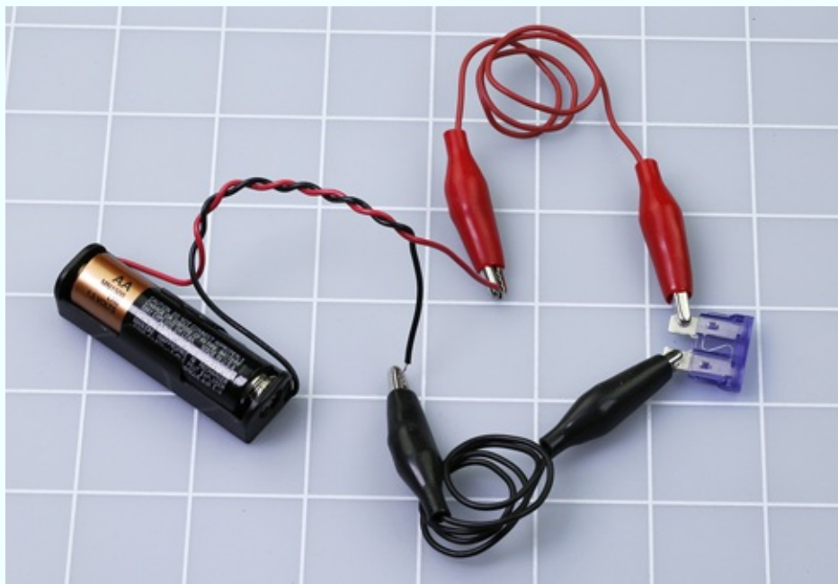
Figure 1-35. How to short out an automotive fuse.
