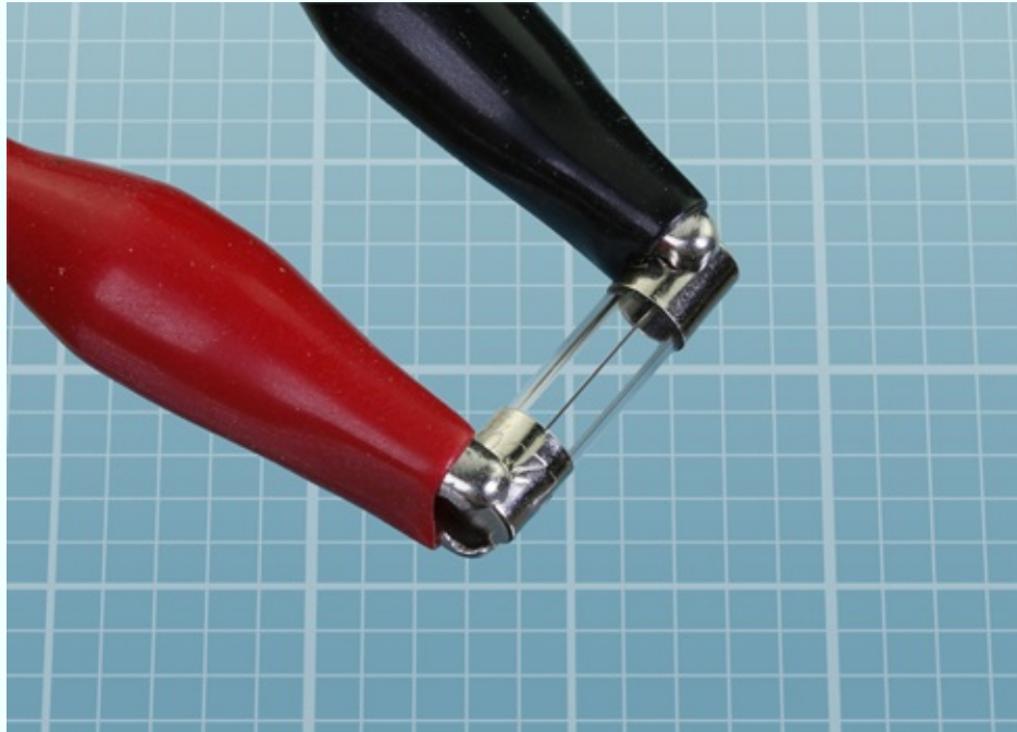
Figure 1-36. How to apply your test leads to a small cartridge fuse.
