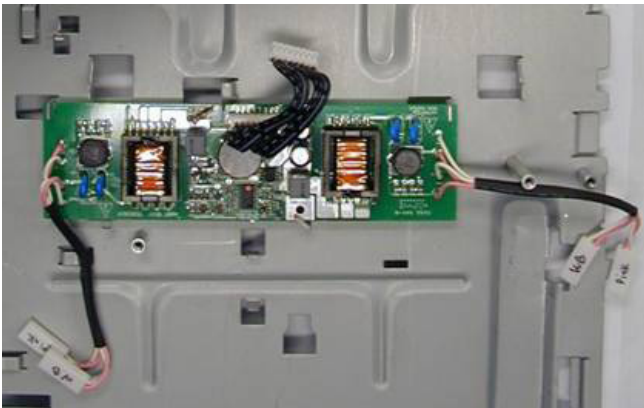
Fig.9 Plaqueta inverter montada
