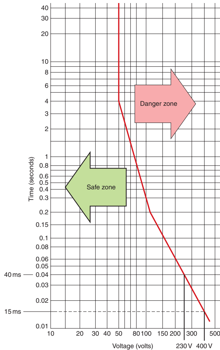
Figure 3.8 Touch voltage curve.
