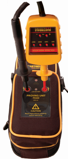
Figure 1.27 Voltage indicator being proved.
