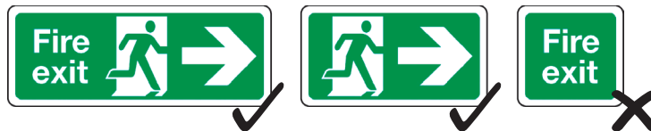
Figure 1.7 Text-only safety signs do not comply.
