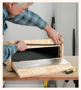
Apply weatherseal around the edges of the hinged door to make the door airtight.
