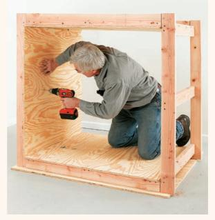
**4** Turn the box on its side. Fasten the plywood sides in place on the long walls, taking care to align corners and edges. Check the box for square as you assemble it.
