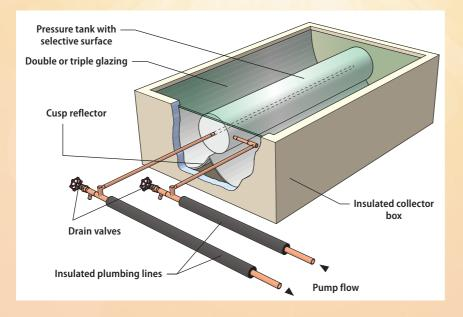
Batch heaters: Instead of pipes, the storage tank itself is mounted outside in a large, insulated heat collector box. It can be mounted above or below the water heater, because pressurized house water flows through it whenever hot water is called for. Batch heaters are sold commercially and can also be made from scratch by a resourceful homeowner, but like the thermosyphon system are generally not suitable for cold climates because of the risk of freezing pipes.
