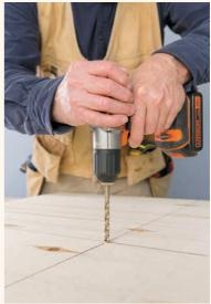
$2^{Flip the plywood base over and draw}_{horizontal and vertical axis lines on the backside. (You will use these lines later to position the leg assembly.) Drill a <math>\%_{e}$ " hole through the center point of the plywood base for installing the threaded quide rod later.
