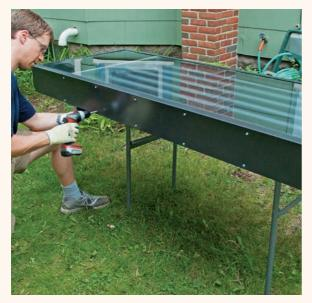
13 Attach the casing. Work with a local metal shop to bend metal flashing that will wrap your panel box. Attach it around the perimeter of the panel with sheet-metal screws with rubber washer heads. *TIP: Be careful when working around the plenum ductwork. If you set the unit down on its back side, you will force the plenum up and break the seal around the opening.*
