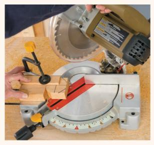
**3** Create the octagonal center block by cutting a 3" square of scrap 2× lumber (1½" thick). Mark the center point by drawing diagonals, then draw a horizontal-vertical axis, as with the plywood base. Make a mark  $\frac{5}{8}$ " to both sides of the axis lines, then connect these marks to draw an octagon. Cut off the four triangular corners along these lines. Drill a  $\frac{5}{16}$ " hole through the center point to complete the block.
