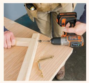
$12^{\text{Construct the leg assembly by cutting two 2" \times 2" legs to} \\ 12^{\text{Length at 22", mitering the top ends at 45°. Cut two cross} \\ \text{pieces at 17". Position the cross pieces between the legs, 3" from the ends of the legs. Drill countersunk pilot holes and join the pieces with two screws.}$
