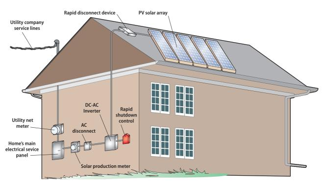
Standard grid-tied systems use the utility grid for "storing" excess power produced by the solar array. A utility production meter keeps track of all solar production and is used to calculate solar renewable energy credits (SRECs), where available.
