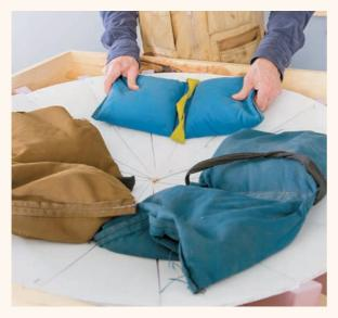
**9** Trace 16 panels onto corrugated plastic, making sure the long sides of the panels are perpendicular to the ribs of the corrugation. Cut out the pieces with a utility knife. Apply thin, wavy beads of construction adhesive to the ribs and apply the panels to the ribs, pressing them down to follow the rib curve. Weigh down the panels with bags of sand, rice, or similar material until the adhesive has set.
