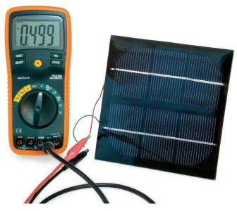
A multimeter is a good diagnostic tool for checking a photovoltaic module to ensure it is working properly. It also allows you to check the power generated at different angles and locations.
