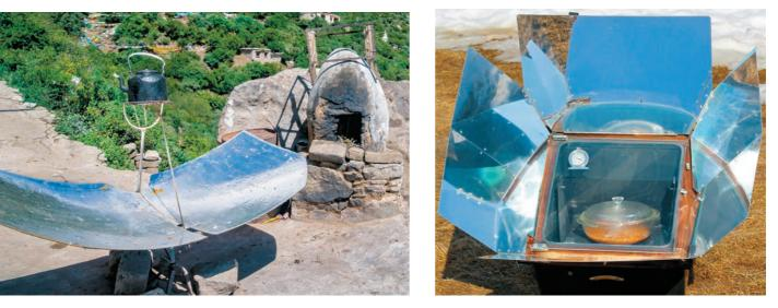
Heat fast, cook slow: A dish-type or parabolic solar cooker (left) creates a focused point of intense heat that can ignite paper in a matter of seconds or, more usefully, heat water or cook food relatively quickly. Cooking in a heat-trapping solar oven (right) is an all-day affair, but even homemade units can reach temperatures upwards of 300°F.
