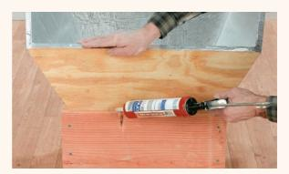
13 Caulk the joint between the angled top and the base with clear, 100% silicone caulk. Set a wire rack inside the oven to keep the cooking pot slightly elevated and allow airflow beneath it.
