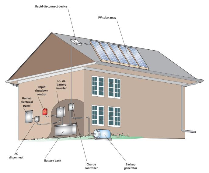
Off-grid systems are self-sufficient and have no connection to the power company. Daily household electricity comes from power stored in the battery bank, but a generator can provide backup power when the battery supply is low.
