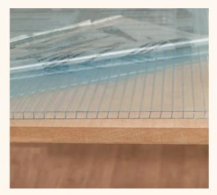
11 The vertical ribs add strength and insulation value to lightweight doublewall polycarbonate, and the two layers help it resist fogging. Cover the top end with waterproof tape and the bottom end with a permeable tape that keeps bugs out.
