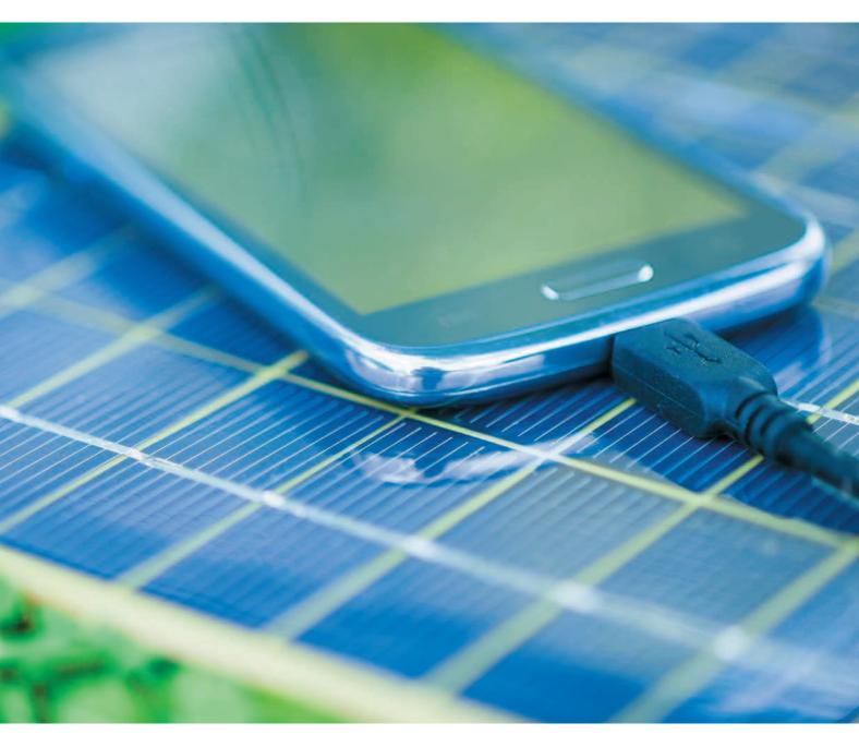
Cell phone chargers are small and lightweight, and generally produce 5 watts or less of power. A basic solar module such as this doesn't store power—it will only charge the cell phone when the sun is out.
