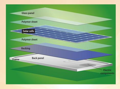
Solar modules are relatively simple pieces of equipment. They are housed within a metal frame, usually aluminum, that frames a back panel to which the electric components are attached. A rigid backing material is at the bottom of the configuration. The solar cells are sandwiched between two polymer sheets that are bonded to the backing. The layers are protected with a glass panel on top that is held in place by the frame.
