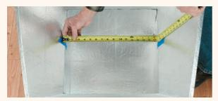
$12^{\text{Take measurements to double-check the glass lid size.}}_{\text{Ideally, the lid will fit in so it comes to rest about 1" above the top opening of the box. As shown here, a <math>\frac{1}{4} \times 17 \times 17$ " piece of tempered glass fits just right. Be sure to order glass with polished edges. You can also just use a clear plastic oven bag instead of the glass. Either will trap heat and speed up the cooking.
