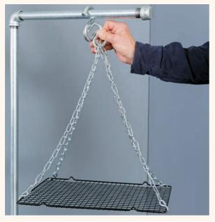
15<sup>Cut</sup> a 14" square of expanded metal using a jigsaw and metal-cutting blade. Use small S-hooks and four 16" lengths of chain to hang the metal square from a single S-hook in the center, then hang the assembly to the large S-hook on the stand with a 12" length of chain. *TIP: You can substitute a heavyduty wire cooling rack for the expanded metal. Choose a size of rack that you won't have to cut down.*
