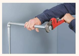
1 Assemble the cooking stand with prethreaded steel pipe and fittings. Thread two 18" pipes into the two side outlets of a 3-way fitting to form the stand base. Tighten the connections with a pipe wrench. Add caps to the ends of the pipes. Thread a 42" pipe into the top outlet of the 3-way, extending up. Add a 90° elbow to the top vertical pipe and then a 20" pipe outward from the elbow. Slip an S-hook onto the 20" pipe, then add a cap.
