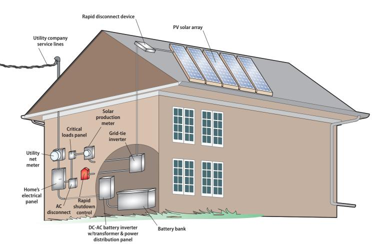
Grid-tied with battery backup systems have many of the same components of both grid-tied and off-grid systems and offer the essential capabilities of both systems. They are suitable only where utility service is readily available.
