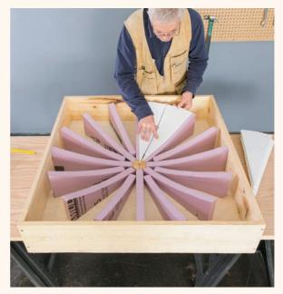
Braw a panel template onto poster board as shown. It is a conical shape with 18½" sides and a 7"-wide base. Cut out the panel template, then test fit it on several pairs of ribs, centering the panel on both ribs. Trim the template as needed for a good fit.
