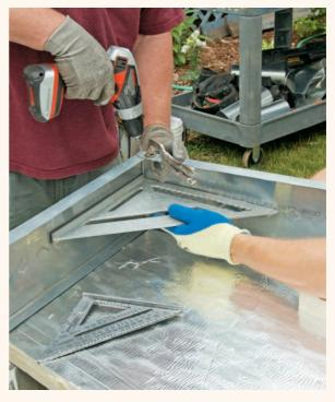
$2^{\text{Drill } \frac{1}{3}^{-}\text{-}dia. \text{ holes in the overlapping top and bottom flanges.}}_{\text{Clamp the corners together before drilling, using a square to make sure the corner forms a 90° angle.}}$
