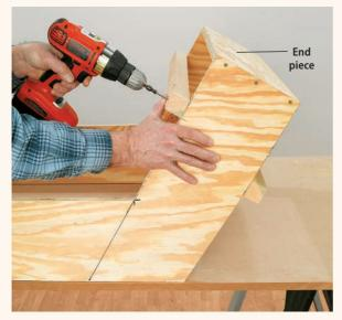
$\label{eq:basic} B_{\rm the window sash in, then subtract 11/2" to get the length of the end pieces, which fit inside the side pieces. Predrill and screw the end pieces in place, then fasten 2 × 2s across the frame at the sash and sill locations.$
