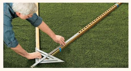
2Cut the pieces to length. Cut the cross supports to match the width of the solar collector or the length between mounting points on the PV panels.
