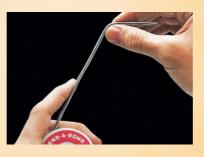
Prepare the wire solder by unwinding 8" to 10" of wire from spool. Bend the first 2" of the wire to a 90° angle.
