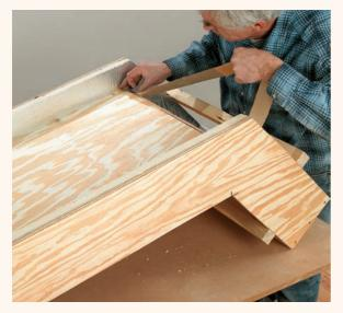
**6** Fasten <sup>1</sup>/<sub>4</sub>" plywood to the top of the 1 × 3 to divide the incoming cool air from the hot air. Leave a 3" gap at the lower end of the plywood for air flow. Butt the two pieces of plywood together at the bend, then cover the small gap with a double layer of aluminum tape. Caulk the gaps at the end and at the corners of the insulation.
