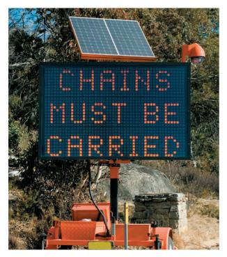
Solar power road signs are a common sight on highways. The light is plugged into a battery, which stores power produced by the PV panel. A charge controller keeps the battery from overcharging.
