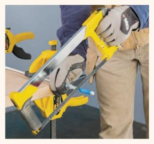
1 Mark a length of  $\frac{5}{6}$  "threaded rod at 22". Thread two nuts onto the rod so they are about 18" from one end and both inside of the 22" mark. Cut the rod at the mark, using a hacksaw. Place a washer over the rod end, and insert it through the hole in the dish's center block, so the rod projects up out of the bottom of the reflective dish. Secure the rod on the backside of the plywood base with another washer and nut.
