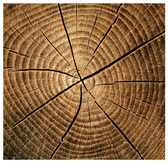
Up to half the weight of a freshly cut tree may be water, and as this water evaporates the wood shrinks, cracks, and warps. Controlled drying of wood can minimize these problems and produce a larger number of solid, furniture-grade boards.
