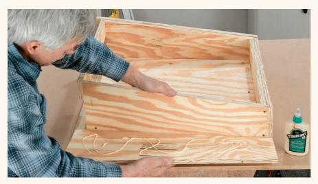
Glue and screw the remaining front and side pieces on, using clamps to hold them together as you predrill and screw. Use 1¼" screws to laminate the pieces together and 2" screws to join the corners.
