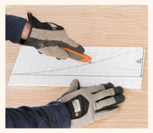
**5** Create a rib template on poster board, enlarging the template to a full-size grid, as shown. The curve starts with a ½" increment because the first 1½" of the parabola is essentially flat (horizontal) and will be taken up by the octagonal center block. Lay out the curve by making a mark at each vertical line, using the dimensions given. Connect the marks with a smooth, curving line to draw the parabola. Cut out the poster board template with scissors or a utility knife.
