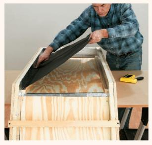
8 Cut two <sup>3</sup>4" nailers an inch shorter than the plywood divider, then fasten them to the plywood and the 1 × 3 to create an air channel above and below the heat-absorbing aluminum. Cut the aluminum to fit across the box, then attach it to the nailers with stainless-steel staples or ½" sheet-metal screws. NOTE: We used a thick, pre-painted aluminum sheet that's available online. If you use aluminum coil stock, paint it black after installing it. See Resources on page 186.
