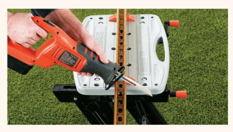
**3** Cut two additional pieces of strut to 4" less than the length of the expandable brace. Cut the expandable brace in half, then bolt both halves to the long center leg with four bolts. To expand the brace to the fall or winter position, just remove the bolts on one side, push the frame up, and then bolt the pieces back together. NOTE: Solar collectors usually stay in a fixed position year round, while PV panels benefit from being moved to summer and winter positions.
