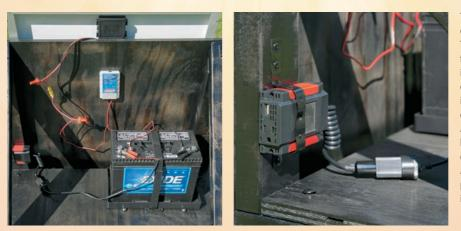
The circuit for a simple solar charging station is fairly basic. The electrical charge comes form the module, through an inline fuse and enters the charge controller. The charge controller is connected to the terminals of a deep-cycle, 12-volt battery. A power lead from a cigarettelighter style DC plug goes to the output terminal on the battery. An AC inverter containing an AC plug and a USB port is plugged into the DC plug.
