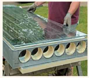
12<sup>Affix</sup> the glass top. First, double-check that all openings in the panel are adequately sealed and insulated. Then, line the tops of the steel stud frame with foam closed-cell gasket tape. Carefully position the glass on top of the gasket tape, lined up ½" from the outside of the frame on all sides. Then, position foam closed-cell gasket tape around the perimeter of the top of the glass panel.
