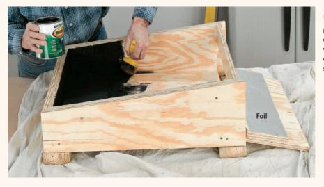
6 Paint the inside of the box with black high-temperature paint. Cover the back and the door with reflective foil glued with contact cement. Let the paint dry for several days so that all the solvents evaporate off.
