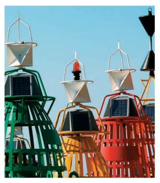
Buoy lights are a perfect use for a solar panel and battery. No other power source comes close to working as well and as cheaply for this application.
