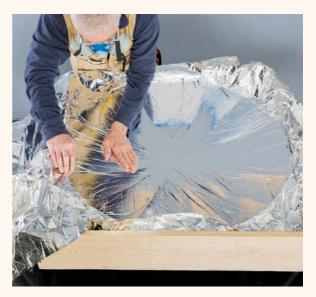
**1** Ospray the dish surface with spray adhesive, then carefully lay a sheet of Mylar over the dish. Smooth the center area down, then work outward, spraying and smoothing as you go. Your goal is the smoothest possible reflective surface. Trim away the excess Mylar.
