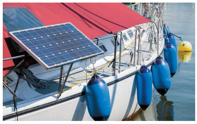
Rigid modules can be mounted on the pushpits at the side or end of a boat or overhead on a pole system. A simple pivot mechanism helps maximize production and allows the modules to swing down close to the boat when they're not needed.
