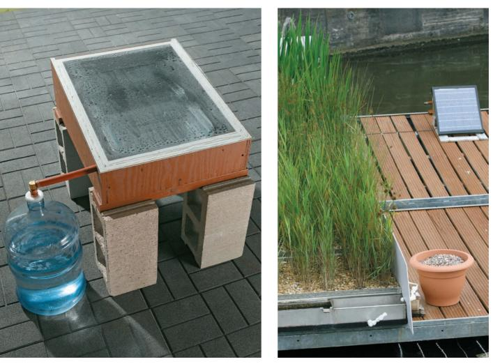
Purify and filter water: A solar still (left) works just fine to distill and purify water for modest consumption. A solar-powered pump (right) also may be used to filter water in off-the-grid locales.
