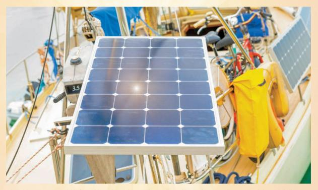
Adjustable mounts are available for sizable rigid modules as well as small portable panels. Mounts that rotate and tilt (or use ball joints for infinite adjustment) are the best for maximizing capture throughout the day.
