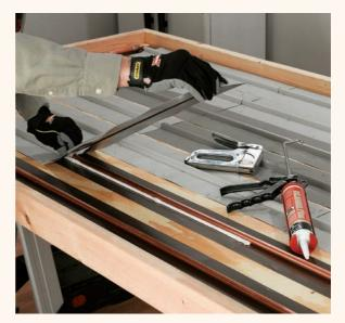
**11** Fasten the manifold in place with copper pipe straps, equidistant from the edges. Spread a bead of silicone caulk on both sides of the copper pipe to fill the void along the bottom edge, then push the aluminum fin sections over the pipe and staple or screw them down as close as possible to the pipe. (The silicone helps to transfer heat from the fin to the copper.) Butt the fins against each other.
