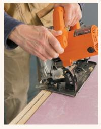
**2** Create the top channel by clamping an 8' 2 × 2 to a work surface and drawing a centerline down the length of the board. Set a circular saw to cut a  $221/2^{\circ}$ bevel at a depth of  $\frac{3}{4}$ ". Cut along the line, moving the clamps if necessary, to cut at least 78" of channel. Test-fit a piece of corrugated plastic sheeting in the channel; it should slide in easily for a snug fit. If necessary, widen the channel as needed by making a second pass with the saw.
