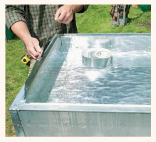
**6** Seal the insulation edges. Place a bead of silicone around the inside corner where the insulation strips and backing panel meet, and then seal with foil tape. Flip the panel over. Place a bead of silicone on the intersection of the  $2 \times 6$  stud flange and the back of the insulation, and seal with foil tape. Conceal any exposed insulation edges with foil tape.
