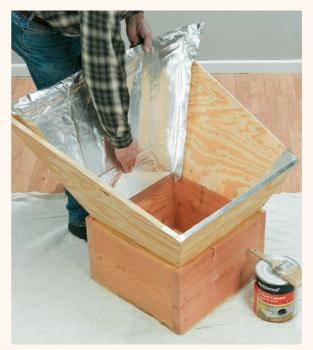
**1** Glue the reflective sheeting inside the base and reflector, overlapping the corners so all bare wood is covered. Use contact cement or silicone caulk to adhere solar foil, and staple the edges to reinforce the glue; use diluted white glue with a paint brush instead of contact cement if you're using aluminum foil. Pull or smooth out the reflective material as much as possible; the smoother the surface is, the better it will reflect light.
