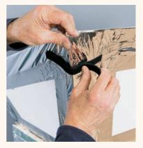
6 Reposition the reflector panels on the oven box and align their edges at the corners. Cut 4"-long strips of hook-and-loop tape and apply one set of strips to secure the two adjacent panels together at each corner, about ½ of the distance up from the oven box. Apply the strips at an angle so they remain flat. Separate the strips and remove the panels for the next step.
