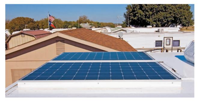
Rigid solar modules are durable and efficient, which makes them a good choice for RVs with a flat roof. Fliexible modules that are very thin ( $\frac{1}{3}$ ) and flex to follow a profile up to 30° make sense atop some RVs that have round roofs.
