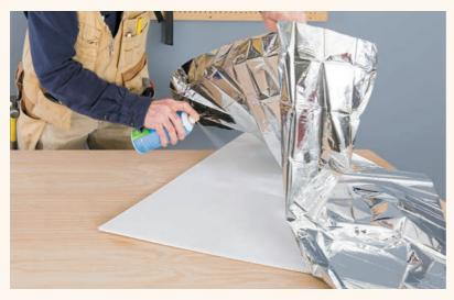
**5** Cut the Mylar sheeting by placing each reflector panel facedown onto the backside of the Mylar and cutting the Mylar around the panel, leaving an ample margin on all sides. Turn the panels face up and coat them with spray adhesive. Apply the Mylar to the panels so it is smooth and flat, then bend the excess over the backside of the panels and glue in place with spray adhesive.
