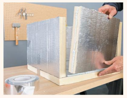
**1** Build the box by cutting two pieces of insulation board to size at  $12 \times 19$ " and two pieces at  $12 \times 16$ " for the four sides, using a utility knife and a yardstick. Cut one piece at  $19 \times 19$ " for the bottom. Glue the sides together over the bottom with foamboard adhesive to form a 19" square. Tape the pieces in place, and let the adhesive cure as directed. *NOTE: Any insulation board you use must be rated for temperatures higher than 450°F.*
