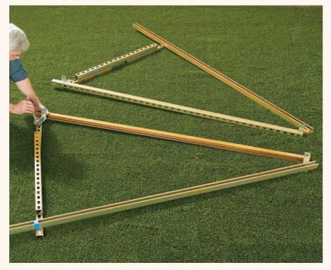
Bolt the brackets and struts together, but don't join the two sides yet. Join the pieces at the base with hinges, or just use an L-bracket with a bolt as the pivot, as we did.
