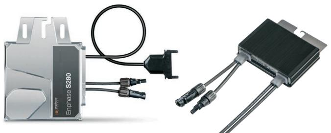
Micro-inverters are installed onto the module or the module mounting rack, then are connected to a cable (called a trunk cable) to form a branch circuit. A PV array may have one or more branch circuits, and each is joined to a junction box mounted to the module racking. *Enphase*
