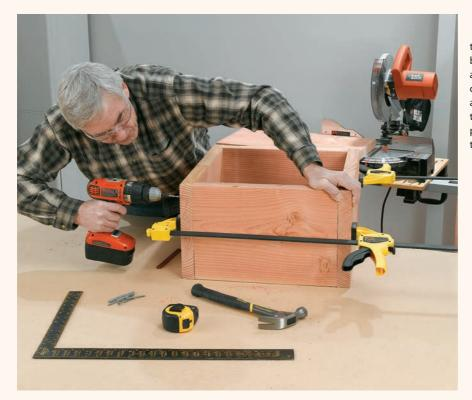
$1 \begin{array}{l} \text{Cut the four } 2 \times 12 \text{ base} \\ \text{pieces to length according} \\ \text{to the cutting list. Arrange the} \\ \text{base parts on a flat work surface} \\ \text{and clamp them together in the} \\ \text{correct orientation. Check with} \\ \text{a carpenter's square and adjust} \\ \text{the parts as needed. Then drill} \\ \text{pilot holes and fasten the pieces} \\ \text{together with } 2\frac{1}{2}\text{ deck screws.} \end{array}$
