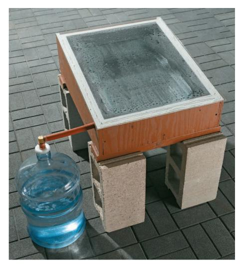
Turn undrinkable water into pure, crystal-clear distilled water with a home-built solar still.
