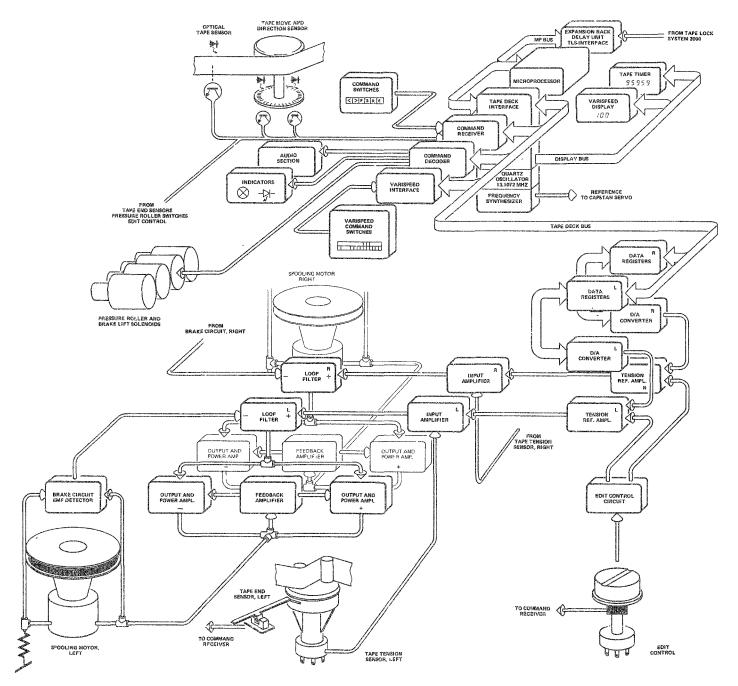
Fig.1 Block diagram showing the spooling motor controls and sensors of a multitrack recorder/reporter (Studer A800).
