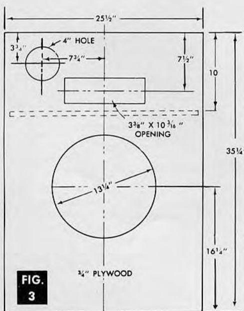
Figure 4. Removable Front Baffle Cutout Details for Build-In Version of the Triplex Reproducer.
