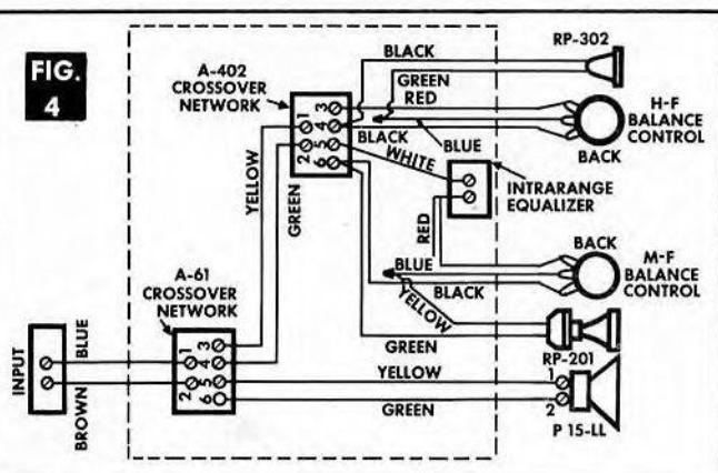
lead of each balance control is spliced to one lead of a driver unit; twist the wire ends tightly and then simply screw on the solderless connectors (Item 13) tightly.
