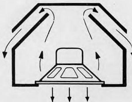
The BASS ULTRAFLEX\* enclosure is a unique Jensen design in which the loudspeaker is attached to the front panel in orthodox fashion but in which the radiation from the back of the speaker is coupled by a large air chamber through ducts or channels to the outside. It can be termed a duct-loaded bass reflex enclosure since the operation is similar but with ducts connecting the opening ports to the inner chamber. These ducts give certain design advantage available in no other way.
