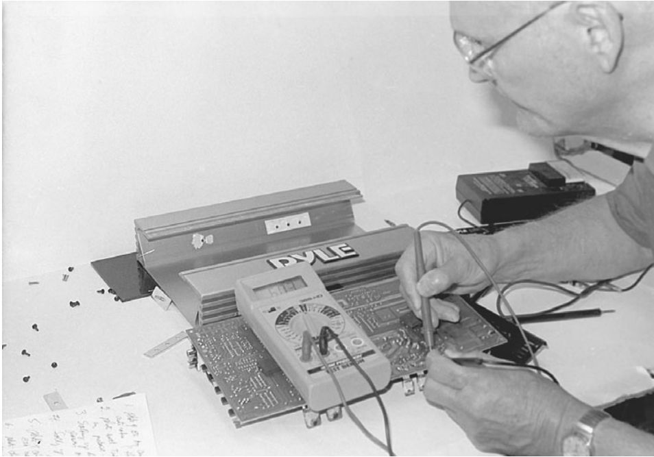
4-20 Checking the power output transistor in a high-powered amplifier.
