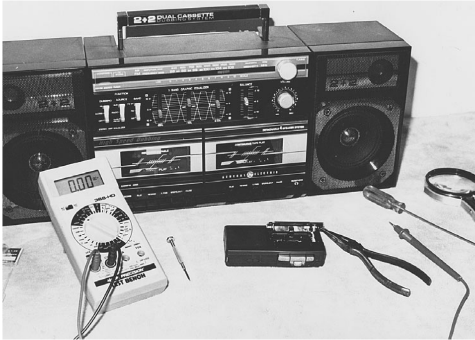
8-13 Locate the power transformer within an AM/FM/MPX cassette player to find the power supply components.
