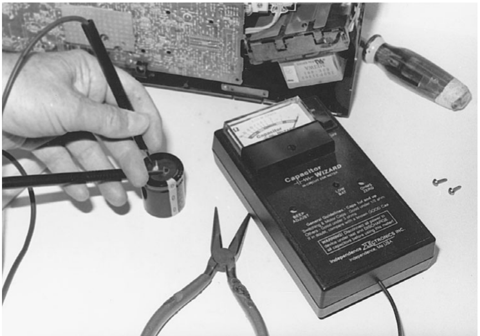
10-20 Check for bad traces and electrolytic capacitors in the front-end circuits with an ESR meter.
