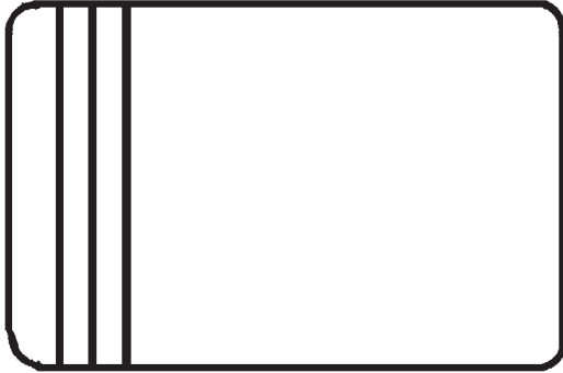
1-12 Black lines to the left of the TV screen are caused by defective parts in the chassis.
