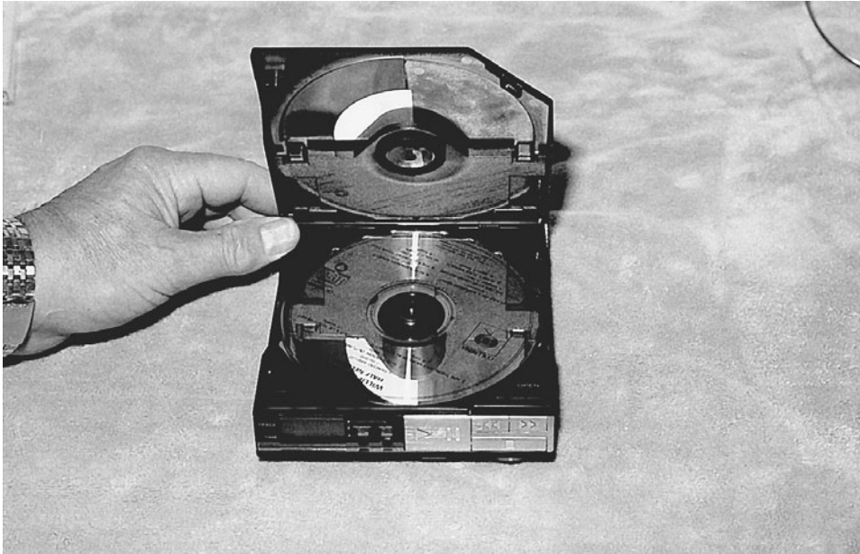
6-8 The top lid must be closed before a portable CD player will operate.
