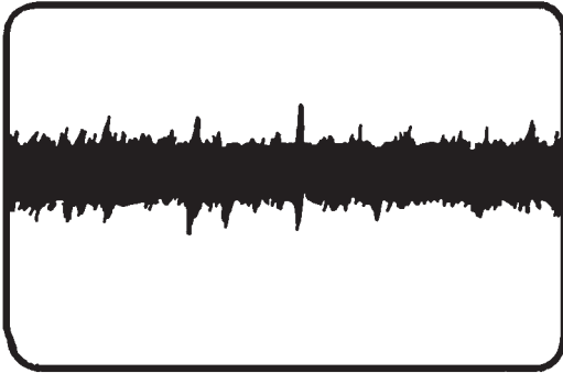
6-40 A focus waveform taken across the focus coil winding.
