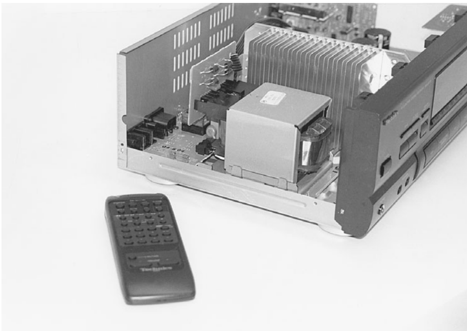
10-37 A simple infrared remote control can operate the tuning, up and down volume of the volume control, and off and on operations in deluxe and surround receivers.
