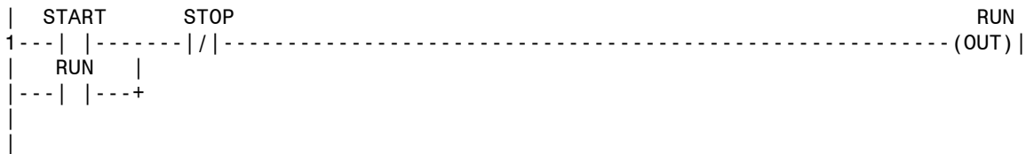
Figure 12-4 - Improved Start/Stop Program With Overriding STOP
