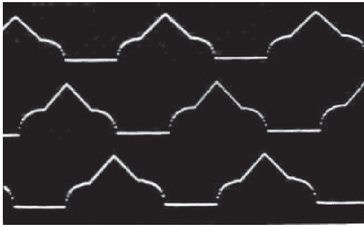
FIGURE 34.94 Micro stepping current references for the VR motor of Fig. 34.93. Stepping rate: 28,800 steps/s., I = 6 A (maximum).
