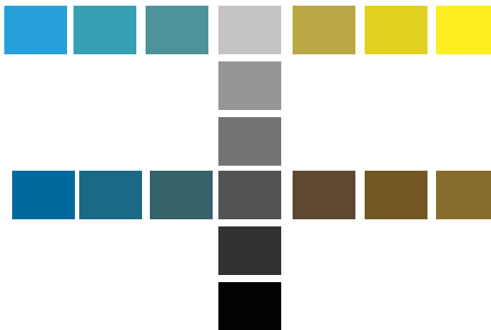
Figure 2.18 Schematic illustration of the general structure of a color space. Lightness increases from black to white from the bottom to the top along the gray lightness scale in the middle. Chroma increases from the gray scale toward the outer colors of
