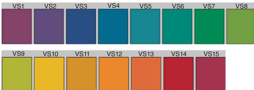
Figure 5.31 Test colors of the CQS method (NIST, USA, version 7.5), VS1-VS15 [30]. Image source: CQS computational spreadsheet (NIST, USA). Not a calibrated reproduction (illustration only).
