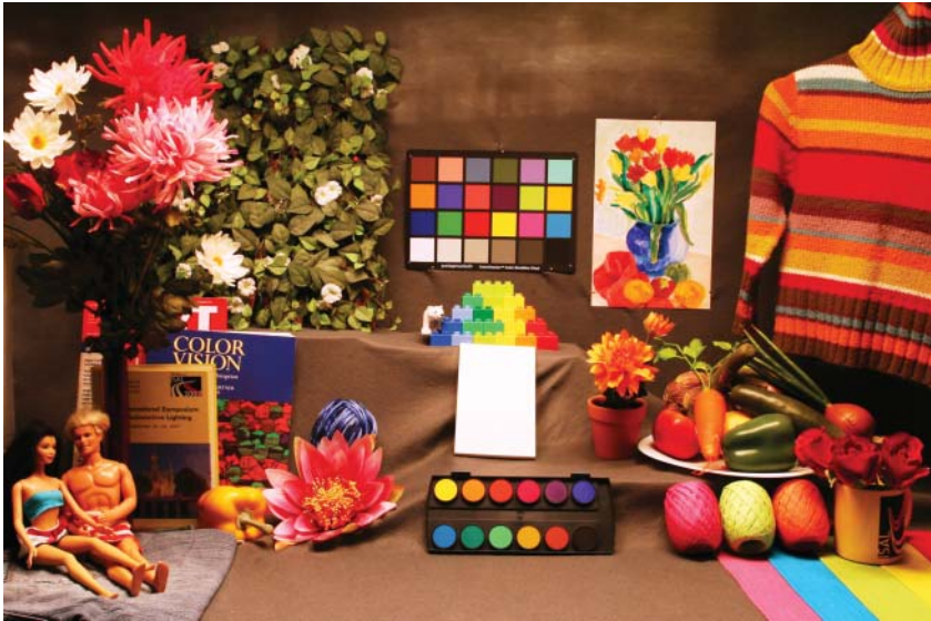
Figure 5.2 Illustration of color quality aspects: a still life or tabletop arrangement of real colored objects in a viewing booth whose light source can be varied. (Reproduced from Ref. [6], with permission from Wiley-VCH.)
