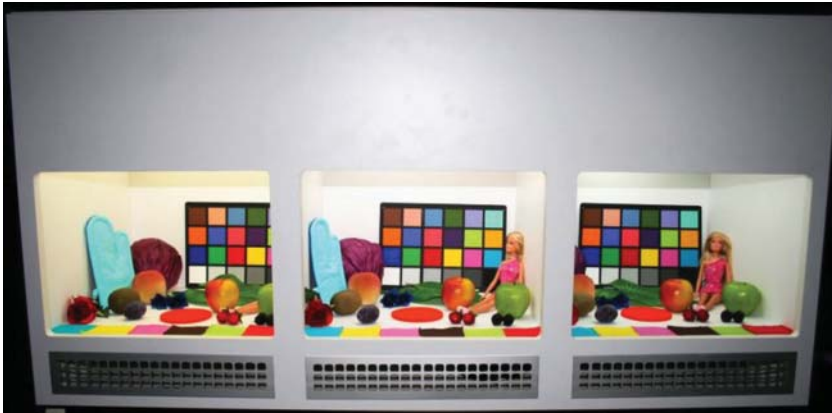
Figure 5.16 Three-chamber viewing booth with the same three set of colored objects. Observers had to assess the similarity of color appearance of the same object (e.g., the red rose) between the left (test A)
