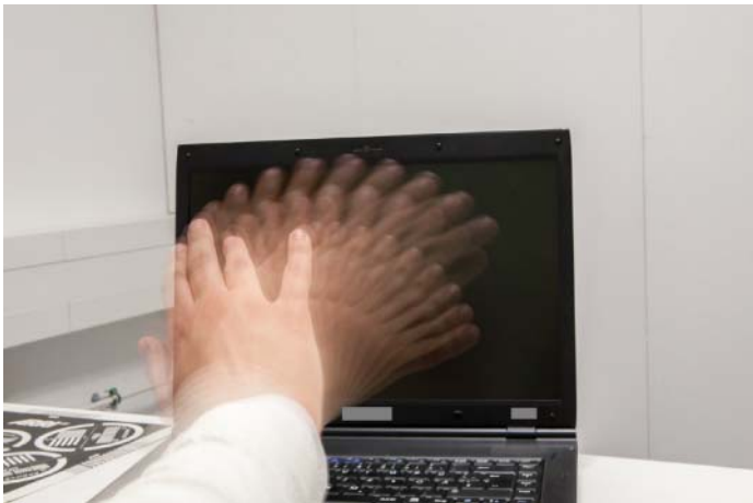
Figure 5.67 Stroboscopic effect of a waved hand in a room illuminated by PWM controlled white LEDs. (Image source: Technische Universität Darmstadt.)
