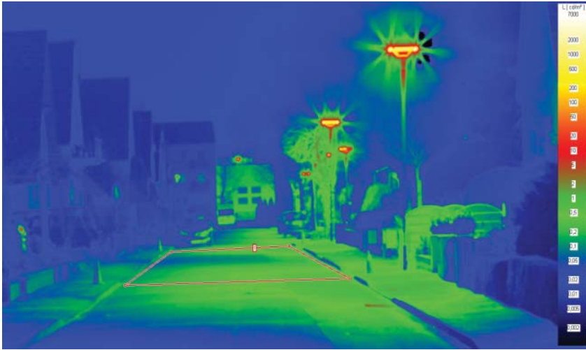
Figure 4.1 Luminance distribution on a road illuminated with LED luminaires. (Image source: Technische Universität Darmstadt.)
