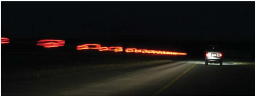
Figure 6.37 Illustration of the bead string artifact on a mesopic background. (Image source: Technische Universität Darmstadt.)
