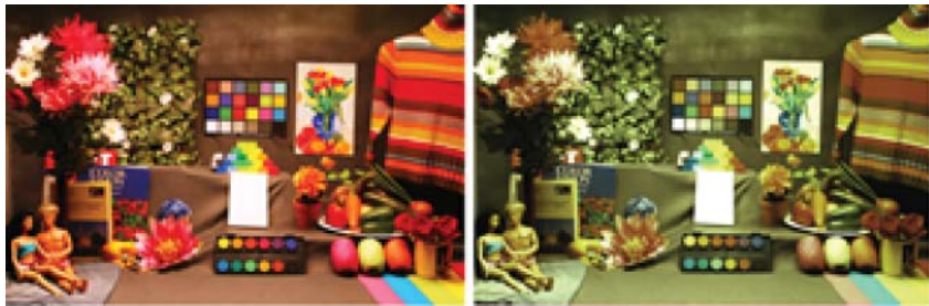
Figure 5.3 Change of color appearance of colored objects if the spectral power distribution of the light source changes following the interaction of light source emission spectra and object reflectance spectra
