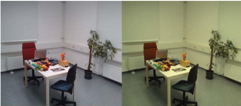
Figure 5.46 Illustration of a room illuminated by different white tones. Left: a white tone acceptable for general lighting; right: not acceptable because of an unexpected greenish shade (e.g., because of the failure
