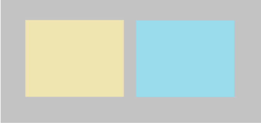
Figure 5.40 Heterochromatic brightness matching experiment. The bluish color stimulus on the right is being changed until the perceived brightness of the two color stimuli becomes the same. The color stimulus on the left (yellowish) remains constant. When
