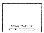
Press both ▼ and ▲ buttons simultaneously to return to the tracking center position.
