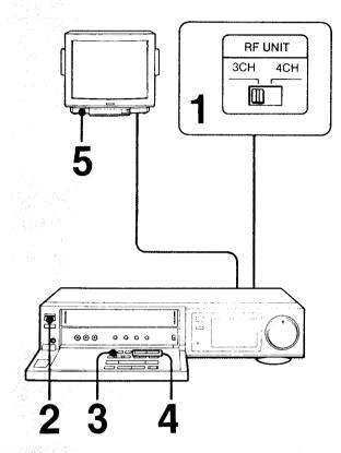
If you have connected your VCR and TV via antenna terminals only, either channel 3 or 4 must be selected on your TV to receive the signal from the VCR. To get the proper RF signal, set the RF UNIT selector on the rear panel of the VCR.
