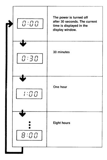
You can change the recording duration with **QUICK TIMER** even during quick timer recording. During recording, the displayed recording duration decreases minute by minute.
