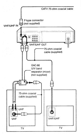
A connecting example is given above, however you should consult your cable company to make sure that the cable is properly connected.
