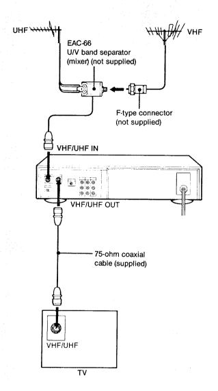
B If the VHF/UHF antenna terminals on the TV are separated
