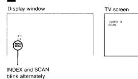
The tape is rewound or rapidly advanced to the next marked index signal, the tape is played back for approximately 10 seconds, and then rewound or advanced to the next index signal.
