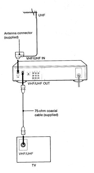
B The VHF/UHF antenna terminals on the TV are separated
