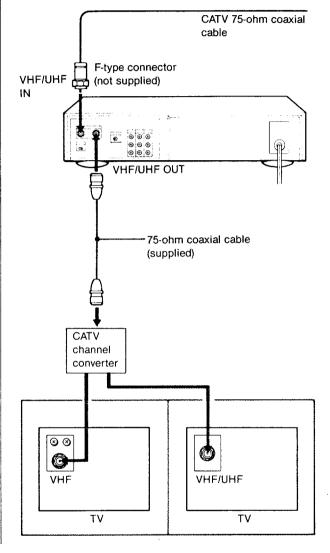
Connect the cable TV channel converter between the TV and the VCR.
