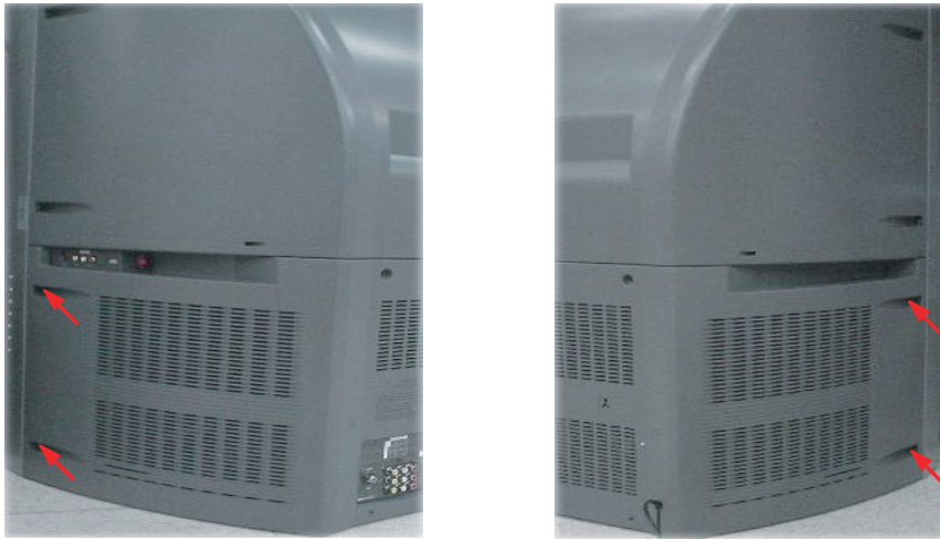
Remove all indicated screws and open the Rear Cover.
