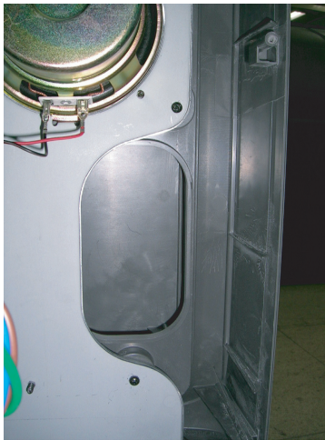
Remove the Screw - Right Back
