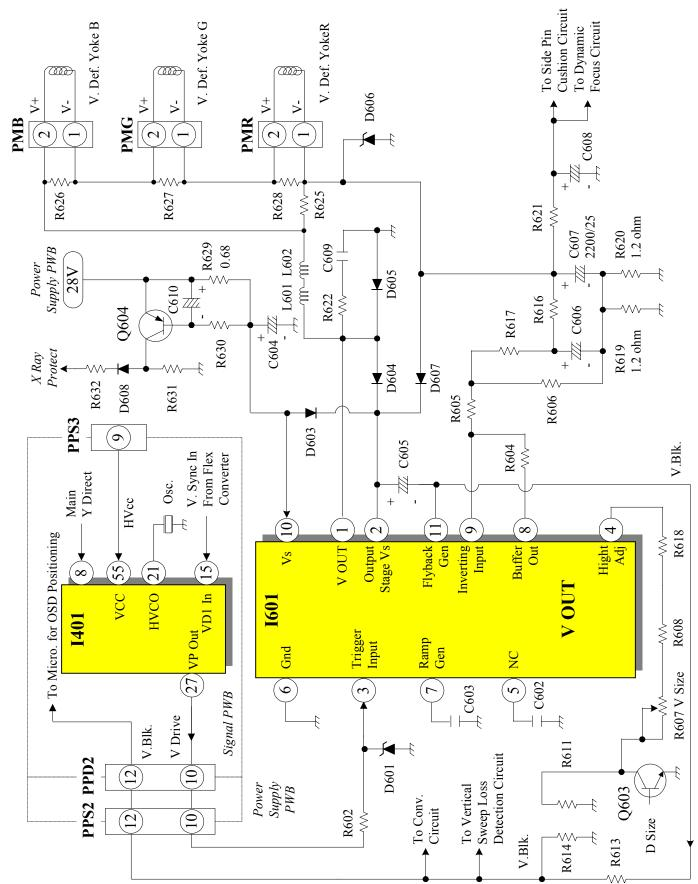
**DP-2X SERIES CHASSIS VERTICAL OUTPUT CIRCUIT**
