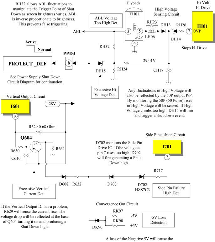
positive 5V to be felt on the anode of DK90 which forward biases the diode and delivers a Shut Down high.
