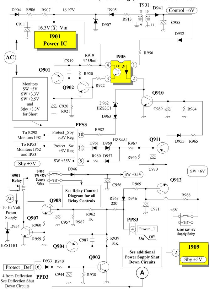
**DP-2X SIGNAL POWER SUPPLY (Low Voltage) SHUT-DOWN CIRCUIT**
