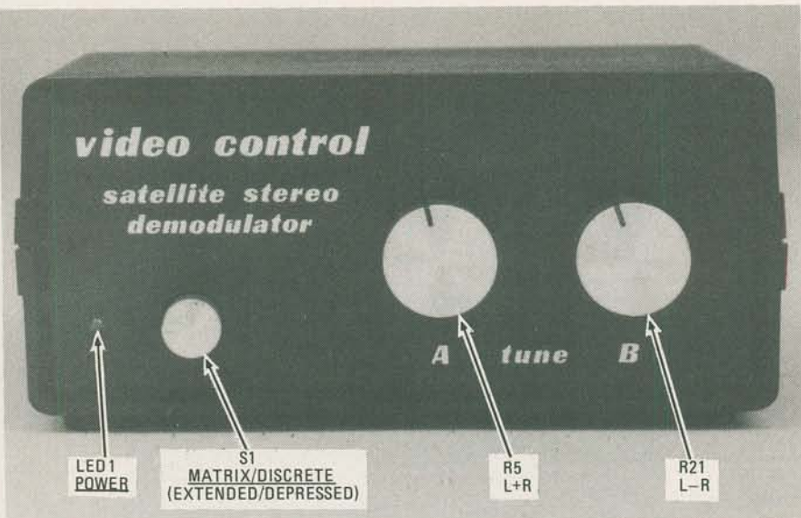
FIG. 9—FRONT-PANEL CONTROLS. To make the unit easier to use, you might want to mark the settings for your favorite transponders around the tuning controls.
