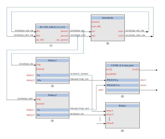
The above diagram shows a simple testing program compiled with the "Logic Master" software. Refer to help documents of the "Logic Master" software for more information.
