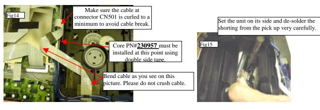
**Solution:** Replace pickup connector cable. "Second time around".
