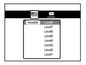
Press the ▲ / ▼ buttons to select the Parental Lock level, then press the ENTER button.
