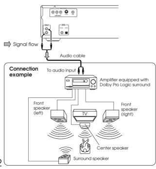
Your DPC-6.1 also supports Dolby Pro Logic Surround. This effect can be obtained in one of two ways; via a digital or an analog connection with an amplifier that supports Dolby Pro Logic Surround (see below).
