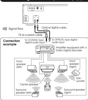
Playback of Dolby Digital-encoded discs requires that you establish a digital connection with the amplifier. The selection of the DPC-6.1's DIGITAL OUTPUT depends on the type of digital input provided on your amplifier. Use either the DIGITAL OUTPUT COAXIAL or OPTICAL connector. See the amplifier's manual for details.
