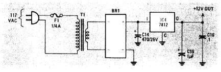
FIG. 5—SIMPLE 12-VOLT POWER SUPPLY is constructed on same PC board as rest of circuit.
