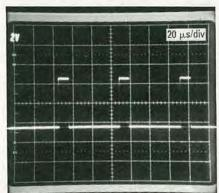
FIG. 19—THE SCOPE DISPLAY should resemble this at IC3 pin 7.
