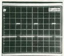
FIG. 20-THE SCOPE DISPLAY AT IC3, pin 10 resembles the display at pin 7.
