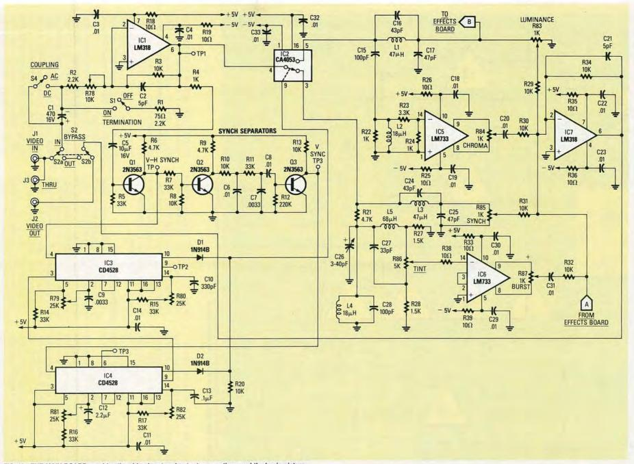
FIG. 10—THE MAIN BOARD provides the video input and output connections and the basic picture processing. Analog switch IC2 separates the sync from the chroma and luminance components.
