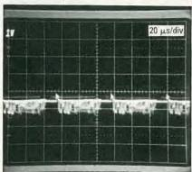
FIG. 23-THERE IS NO SYNC at IC2 pin 5.
