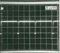
FIG. 17—NEGATIVE PULSES at Q1's collector.
