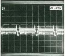
FIG. 25-AN INVERTED VIDEO OUTPUT has the picture information going negative.
