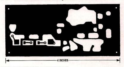
COMPONENT SIDE of the upconverter board.
