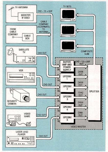
verter and amplifier modules are shown in Fig. 2. The upconverters consist of a preamplifier operating at 60-66 MHz, with 23-dB gain, and a two-pole bandpass filter between the amplifier and mixer. A double-balanced mixer combines the 60-66 MHz (Channel 3) TV signal with a local oscillator (LO). The LO is set to operate at a frequency 60 MHz below the low end of the desired output signal. For example, to obtain an output on Channel 39 (620-626 MHz), the LO must be at 560 MHz.
