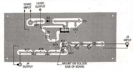
FIG. 6—PARTS-PLACEMENT DIAGRAM for the amplifier/power supply board.
