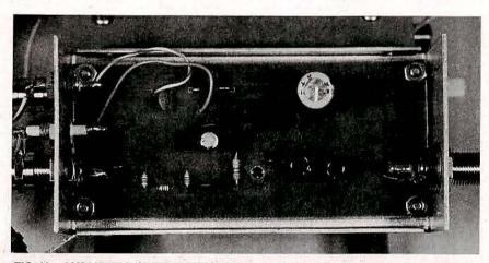
FIG. 10—AMPLIFIER/POWER SUPPLY. This board is mounted in the same type of case as the upconverter modules.
