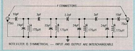
This filter will remove all signals except Channel 3 (or 4) from the output of your cable box.
