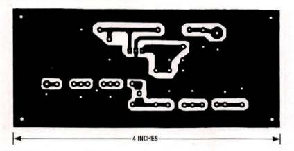
SOLDER SIDE of the amplifier/power supply board.
