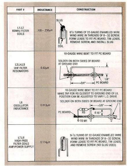
FIG. 7-COILS L1-L7 are made according to these instructions.
