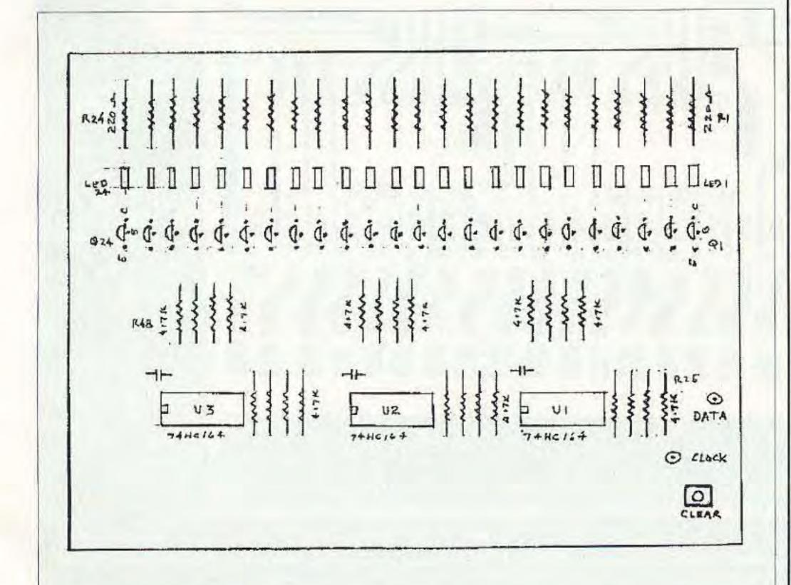
Fig. 3. Component placement for the data receiver.
