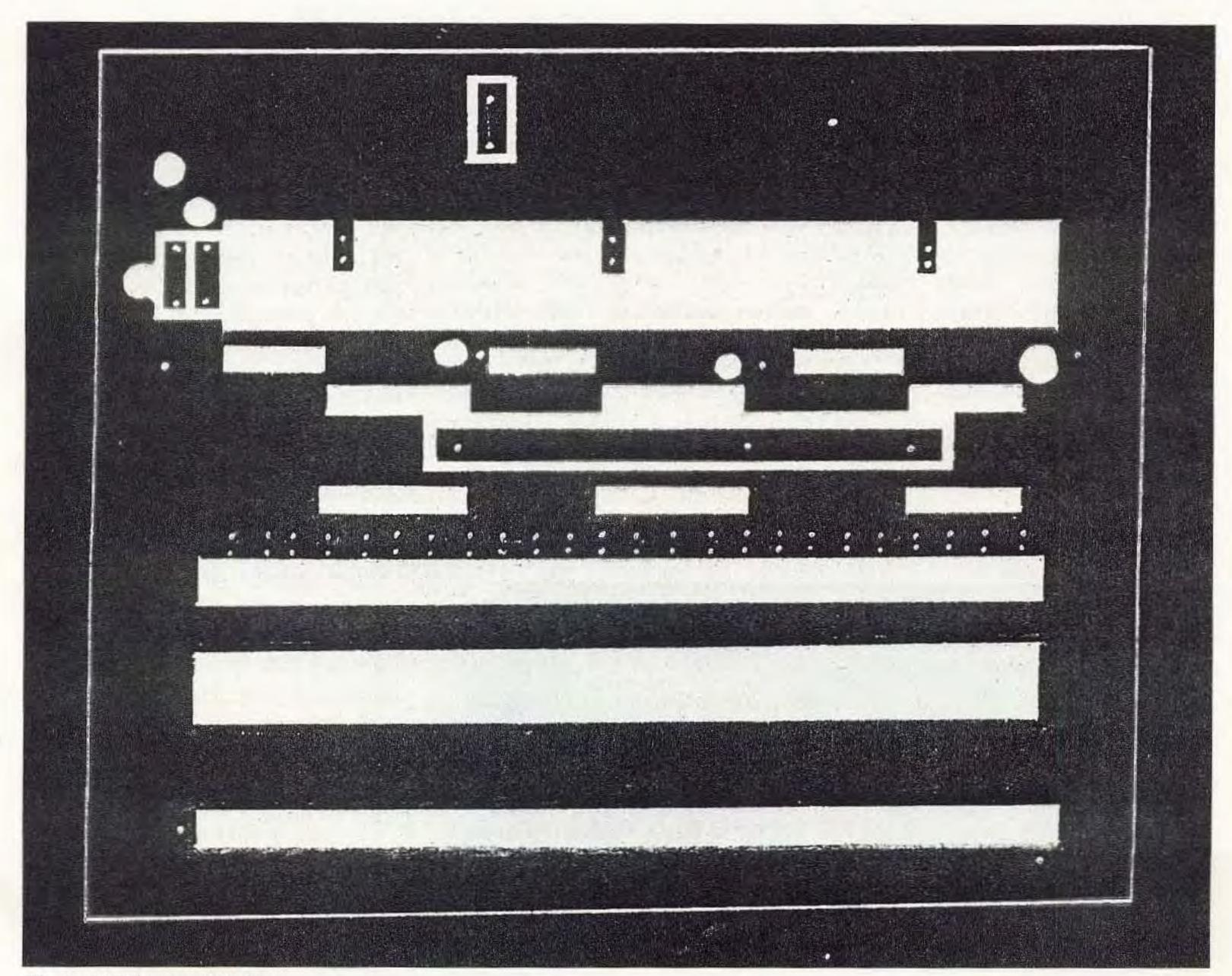
Fig. 5. PCB bottom foil side.
