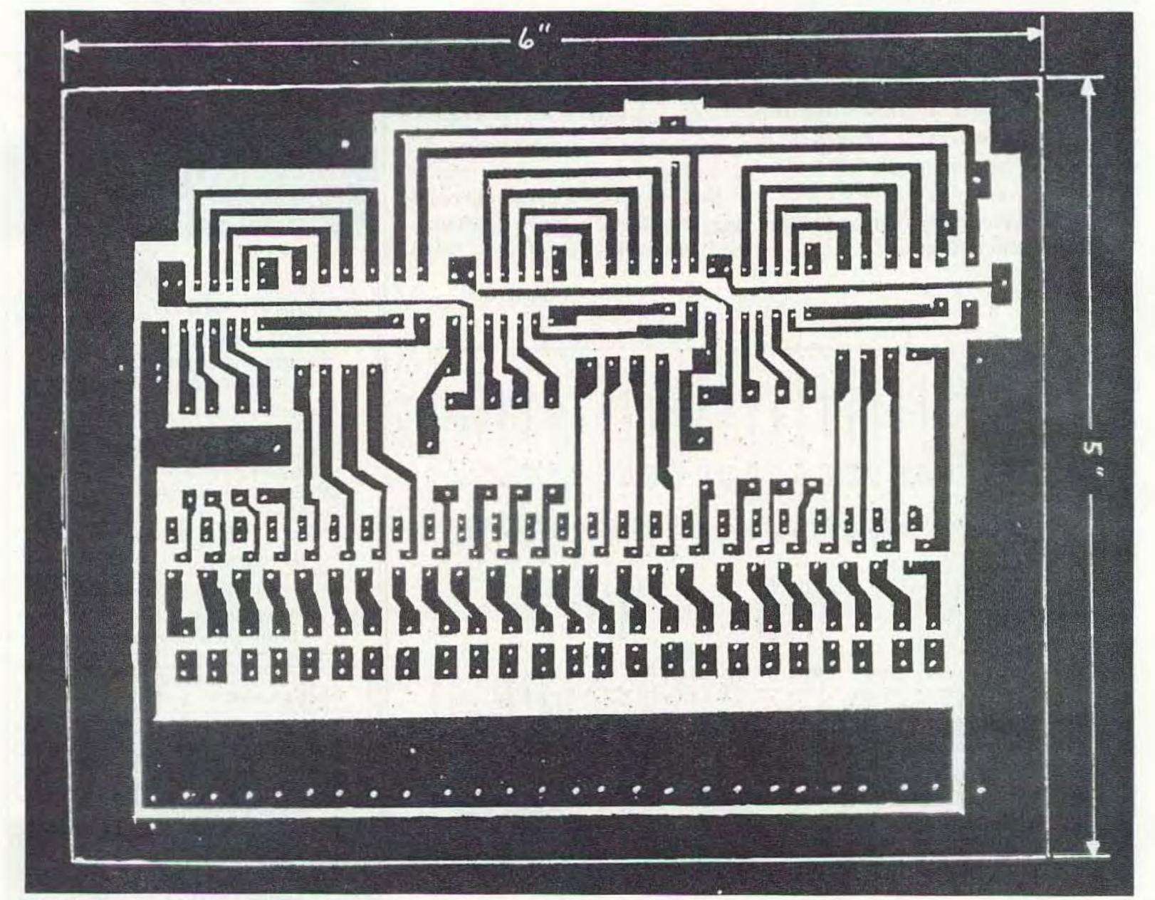
Fig. 4. PCB top foil side.
