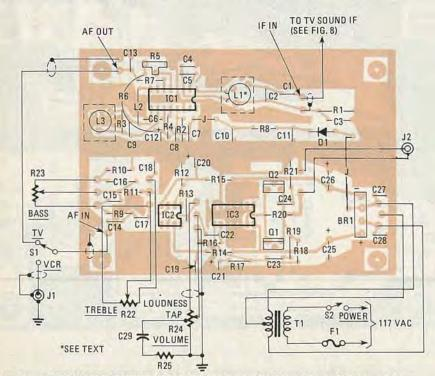
FIG. 4—PARTS-PLACEMENT DIAGRAM. Both on-board and off-board connections are shown.
