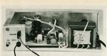
FIG. 7-THE OFF-BOARD components should be mounted before they are wired to the board.
