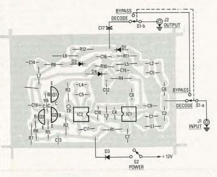
FIG. 7—IF YOU USE THE PC PATTERN shown in PC service, use this diagram when mounting the components.
