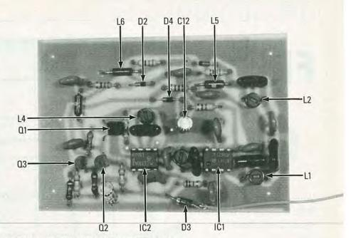
FIG. 8—THE FINISHED OUTBAND DECODER is shown here.
