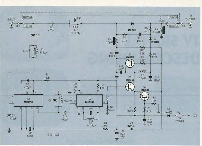
FIG. 6—FOR THE OUTBAND DECODER shown here to work, the cable company must provide at least a 1 millivolt signal. Values for C1–C5 and L1–L4 are found in Table 1.
