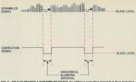
FIG. 2—WE CAN DECODE A SCRAMBLED SIGNAL by adding a correction signal to it, thus restoring the horizontal-blanking pulse to its proper location.
