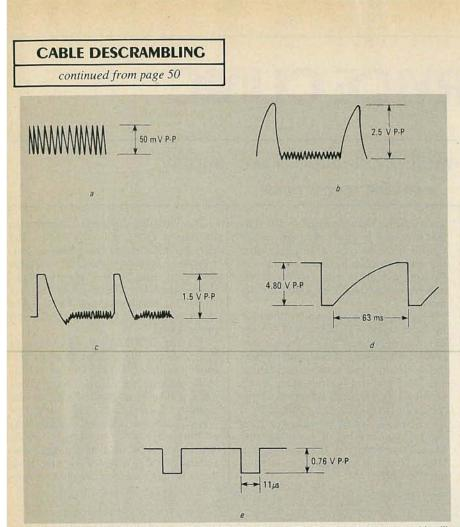
WHEN TESTING THE DECODER, look for the following signals: The input should look something like what's shown in *a*. The signal in *b* should be seen on pin 5 of IC1. The signals in *c* and *d* should be seen at the base and collector of Q3 respectively. The waveform shown in *e* should be seen at the junction of R10 and R11.
