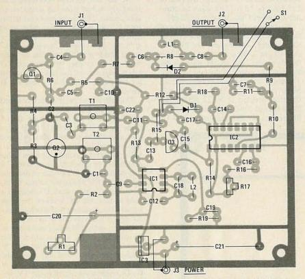
FIG. 7—PARTS-PLACEMENT and off-board connections are shown here. Note that the jacks used depend on your power source and RF connections. (We used a 1/2-inch jack and F-type connectors.)
