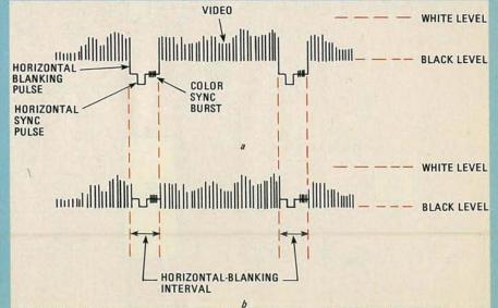
FIG. 1—THE INBAND GATED-SYNC scrambling method moves the horizontal-blanking pulse of a normal signal (a) into the video portion of the signal (b).
