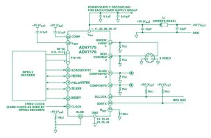
Figure 4. Connection to MPEG decoder.
