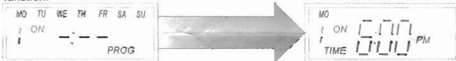
FIG 5: Setting the timer to turn on at 6 PM each Monday for Program 1
