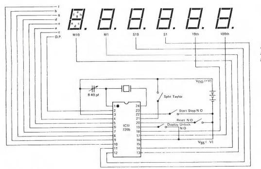
Fig. 1. Circuit for stopwatch using the 7205 chip.
