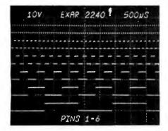
Fig. 2. Output on pins 1 to 6. Scope photos taken with C-59 camera on a Tektronix 7603 scope with 7M13 plug-in readout unit.
