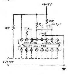
Fig. 1. Schematic of XR-2240 in free-running (astable) mode.
