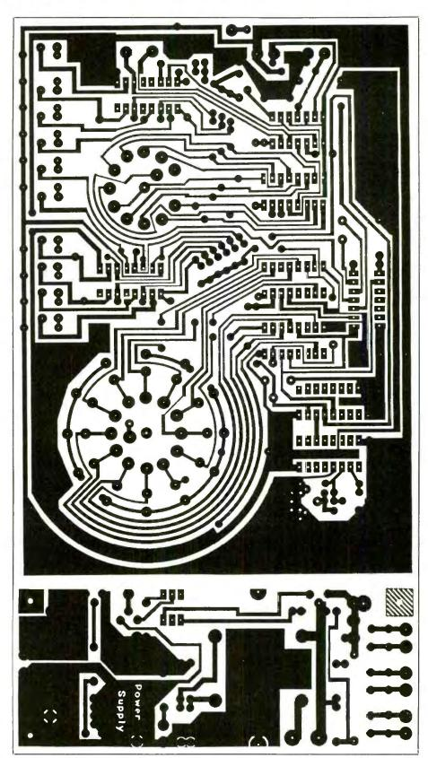
Fig. 5. Actual-size etching and drilling guides for the counter and power-supply/controller printed-circuit boards.
