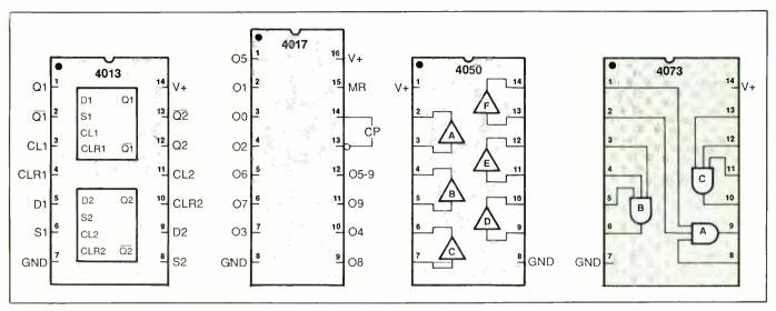
Fig. 2. Pinouts of some 4000-series CMOS ICs used in this project.
