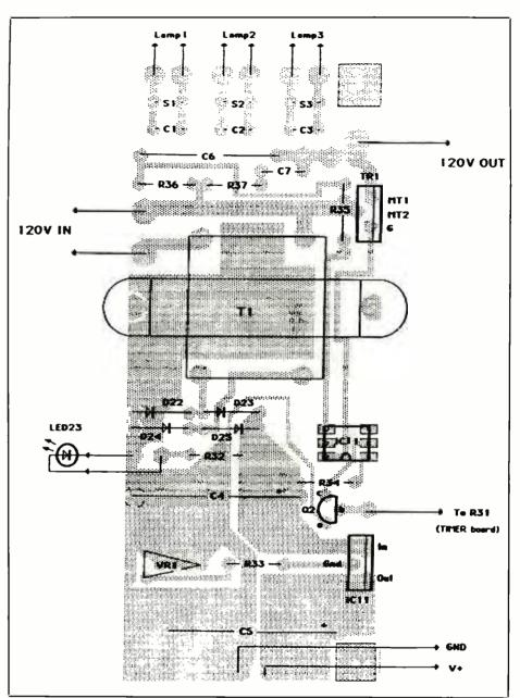
*Fig. 7. Wiring guide for power-supply/controller board.*
