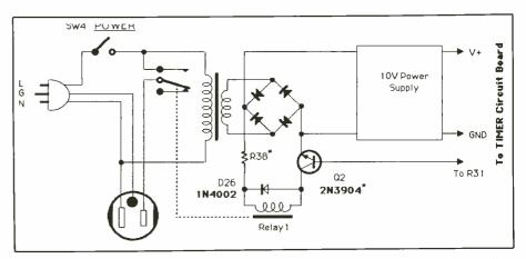
Fig. 4. An alternate controller-circuit arrangement that replaces the triac and its associated components in Fig. 2 with the simpler relay arrangement shown here. The basic power-supply circuitry remains the same.
