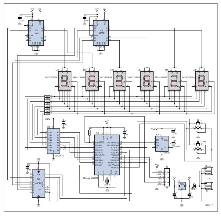
Figure 1. The ATmega168 controls six large 7-segment display characters.
