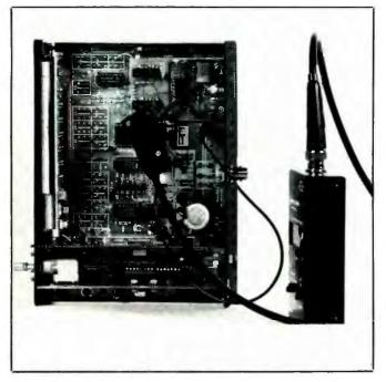
**Direct Probe.** A  $1 \times$ , general-purpose direct probe is used to connect the counter to a crystal oscillator circuit.
