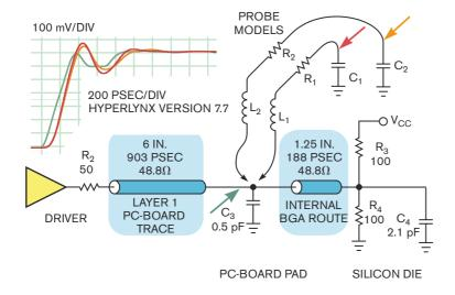
Figure 1 A second probe changes the observed waveform.
