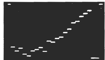
Fig. 14. Typical RTA output on a dc-coupled oscilloscope when "semi-white" noise from an FM tuner is applied to the Analyzer.
