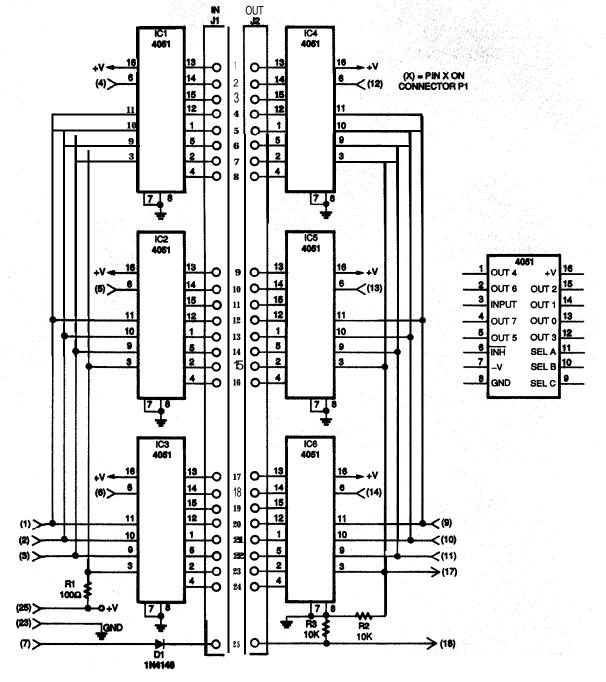
FIG. 3—TO MAKE A PC do continuity testing, the mechanical switches in Fig. 2 must be enplaced with electronic ones. The 4051 contains eight electronic switches.
