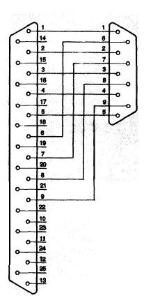
FIG. 5—TO CHECK A DB-9 CABLE, make two adapters and connect them to JI and J2.
