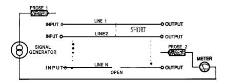
FIG. I-CONTINUITY IS TESTED MANUALLY by providing a test signal at the Input of one wire and then checking each of the outputs for the signal.
