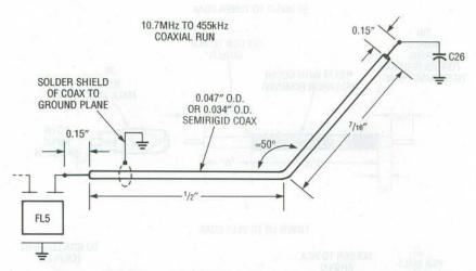
FIG. 13—THE 10.7 MHz TO 455 kHz COAXIAL RUN reduces spurious pickup from the 455-kHz IF.
