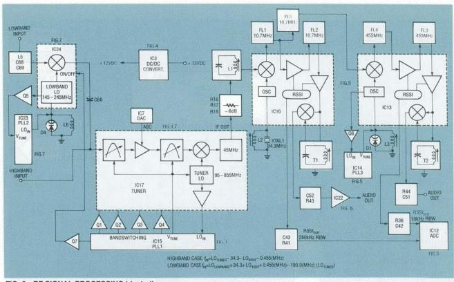
FIG. 6-RF SIGNAL PROCESSING block diagram.
