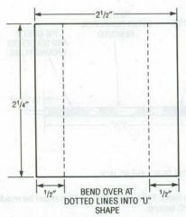
FIG. 19-THE LOWBAND SHIELD is soldered on the top side of the PC board.
