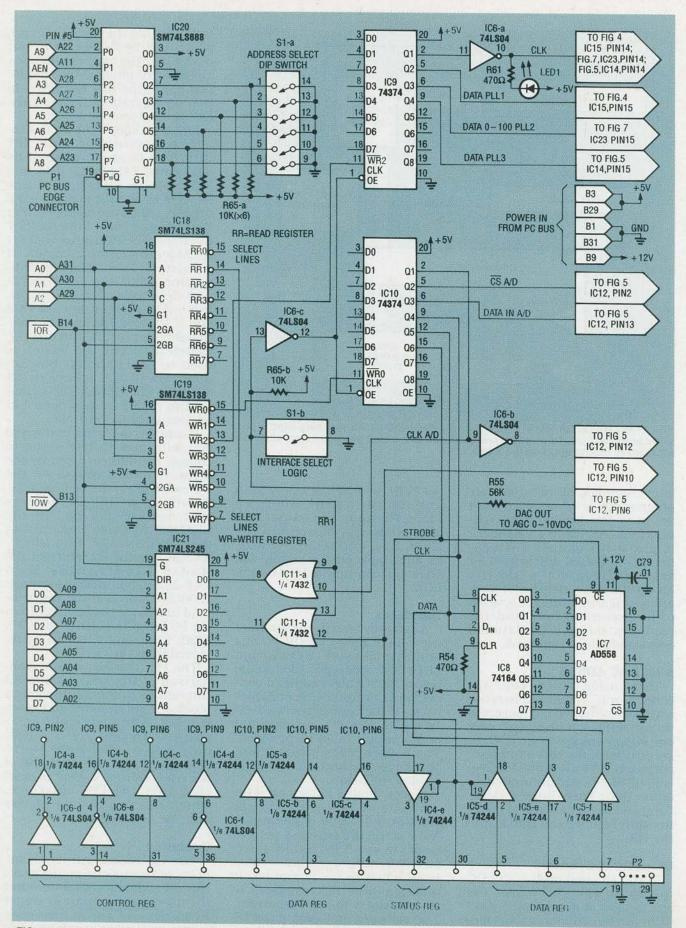
FIG. 10—PC BUS INTERFACE CIRCUITRY. The entire LPT interface is performed by IC4 and IC5. Those two 74LS244's buffer the signals to and from the LPT interface.
