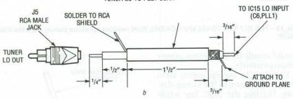
FIG. 15—TWO RG-174 COAX RUNS ARE SHOWN for the RF input to tuner (a) and the tuner LO to the PLL1 (b).
