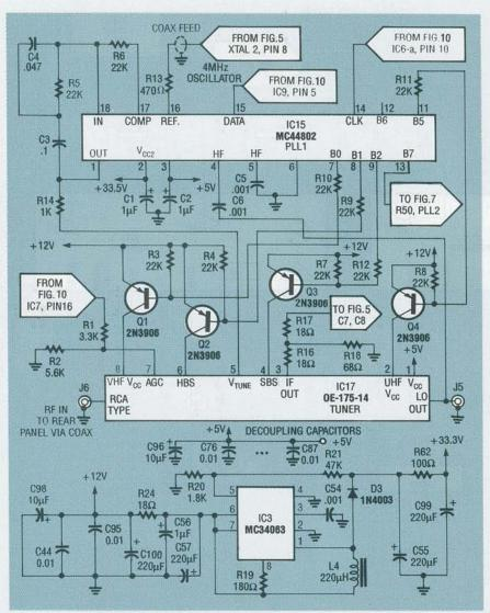
FIG. 4—THE FIRST 45-MHz IF STAGE. The tuner takes highband inputs from 50–810 MHz and converts them to 45 Mhz.
