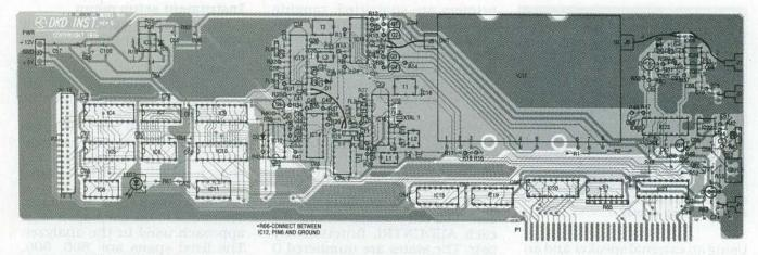
FIG. 12—PARTS PLACEMENT DIAGRAM. Note the location of the four coax runs. Make sure you install all chip capacitors first because of their small size.
