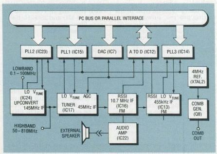
FIG. 3—A BLOCK DIAGRAM OF THE SPECTRUM ANALYZER shows the tuner module, hase-locked loops, receiver blocks, DAC, ADC, and the PC bus connection.
