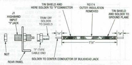
FIG. 17—THE HIGHBAND COAX RUN is shown here. This coax connection must be made before the terminal panel is installed on the PC board.
