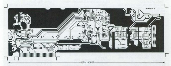
THE SOLDER SIDE of the foil pattern is shown here.
