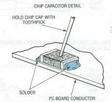
FIG. 14—USE THIS DIAGRAM as a guide to installing the chip capacitors.
