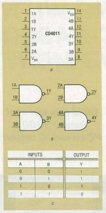
FIG. 1—IC SPECIFICATIONS. It takes a pinout (a), functional diagram (b), and a truth table (c) to fully specify an IC.
