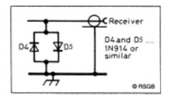
Figure 3 Receiver input protection
