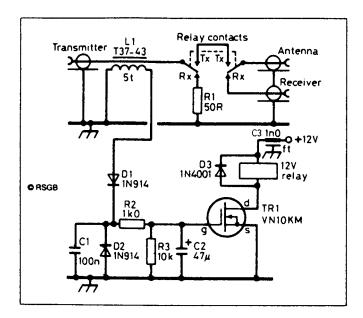
Figure 1 RF activated relay
